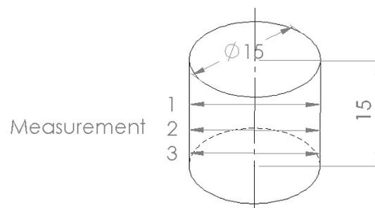
**Figure 6.** Sample model with indication of measurement locations at three levels.
