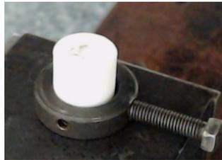
**Figure 7.** Sample clamping during CMM measurements.
