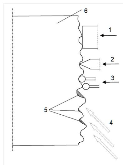
**Figure 5.** An example model of the effect of surface macrostructure on the result of measuring a geometric quantity, 1—the flat tip of a caliper or other contact sensor, 2—the blade of a caliper or other contact sensor, 3—the contact sensors of a measuring machine with a spherical blanket, 4—the light rays of a scanner, 5—the shadow effect from surface irregularities, 6—fragment of the sample.
