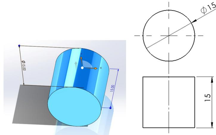
**Figure 1.** 3D CAD model of the sample.
