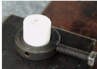
**Figure 7.** Sample clamping during CMM measurements.
