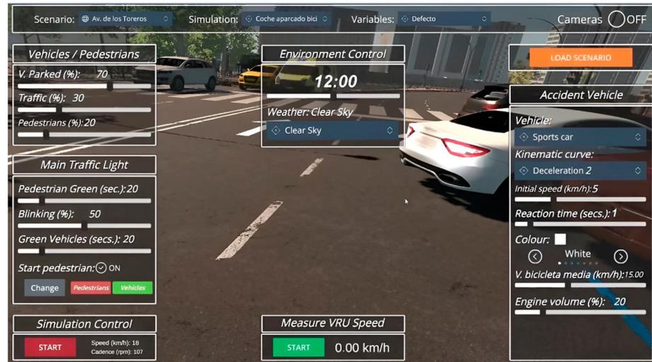
**Figure 9.** User interface of the first-person cyclist view and simulation options of the VR application. Virtual reality simulator interface for one of the accident scenarios.
