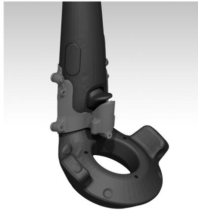
**Figure 5.** 3D reconstruction of the pushbutton mechanism to synchronize the braking of the levers with the virtual bicycle deceleration.
