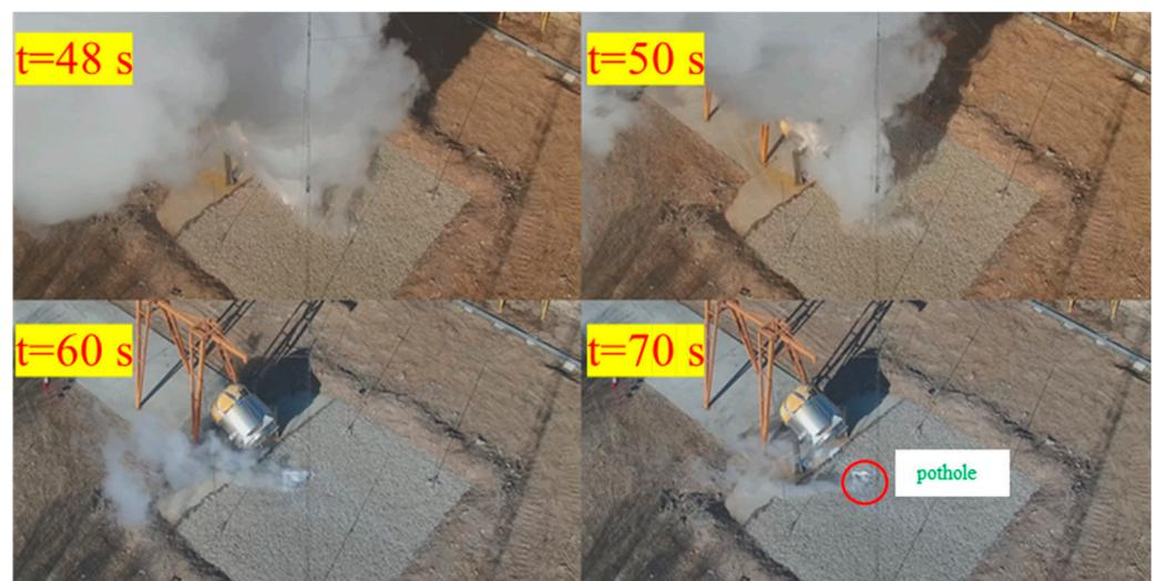
**Figure 7.** The visible cloud behaviors after terminating the release near the ground in Test 8.
