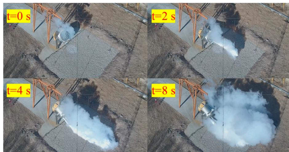
**Figure 5.** The visible cloud behaviors during the release near the ground in Test 8.
