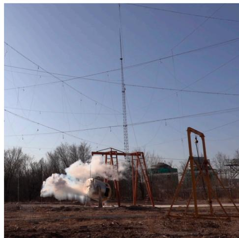
**Figure 1.** The configurations of the liquid hydrogen release experiment.
