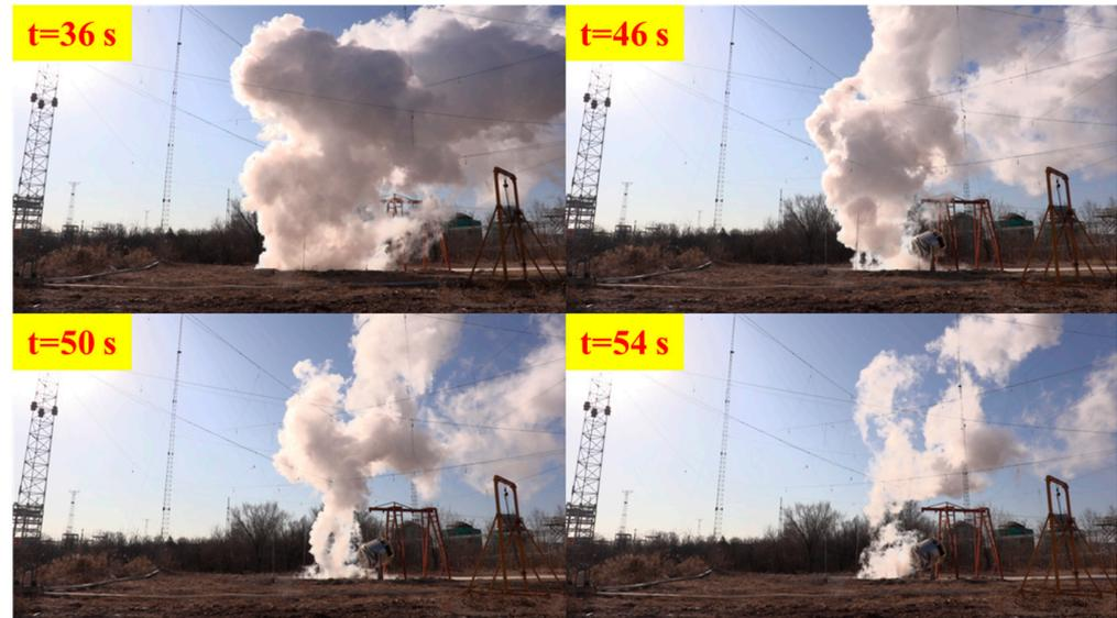
**Figure 8.** The visible cloud behaviors after terminating the release in the atmosphere in Test 8.
