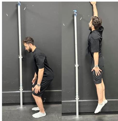
**Figure 3.** Leg power: non-countermovement vertical jump test.
