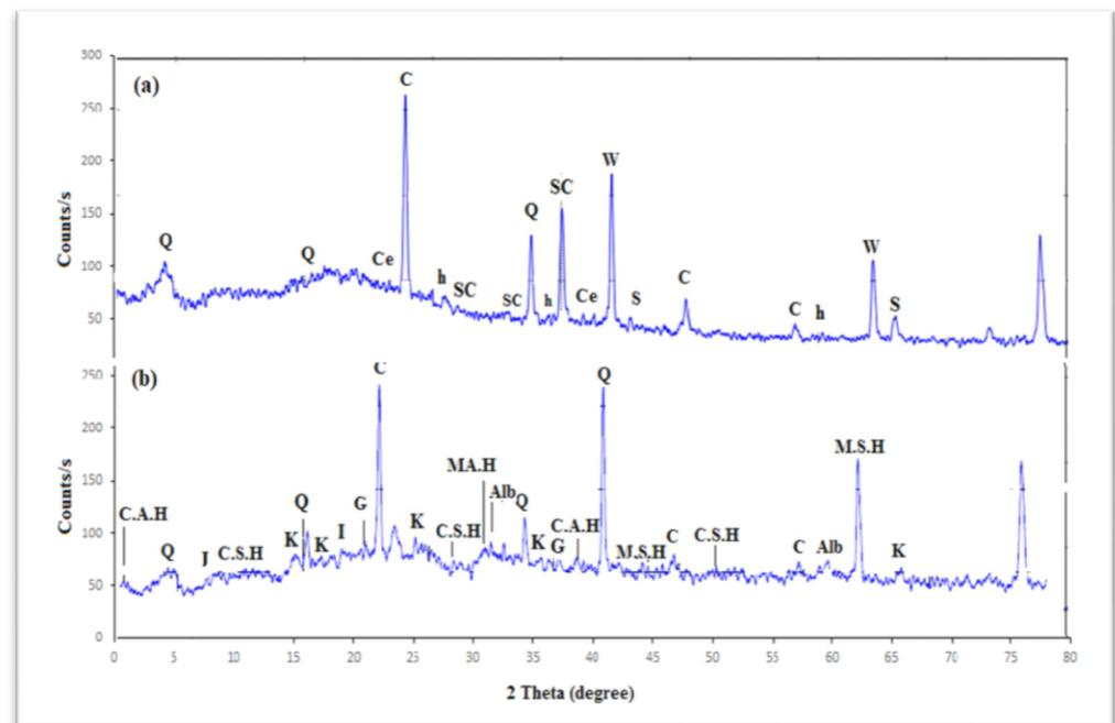
**Figure 4.** (a) X-ray diffraction (XRD) spectrum of nB (Q is quartz; S is sylvite; C is calcite; Ce is cellulose; SC is sodium carbonate; W is whitlockite; and h is hydrozincite). (b) X-ray diffraction (XRD) spectrum of nWTR; (Q is quartz; C is calcite; K is Kaolinite; I is illite; G is goethite; C.A.H is calcium aluminate hydrate; C.S.H is calcium silicate hydrate; M.A.H is magnesium aluminate hydrate; and C.S.H is calcium silicate hydrate).
