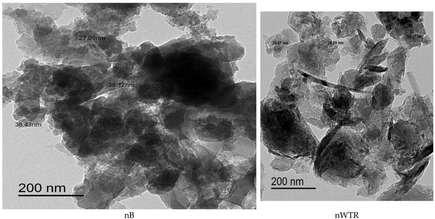
**Figure 2.** Transmission electron microscope (TEM) image for nanobiochar (nB) and nanowater treatment residuals (nWTR).
