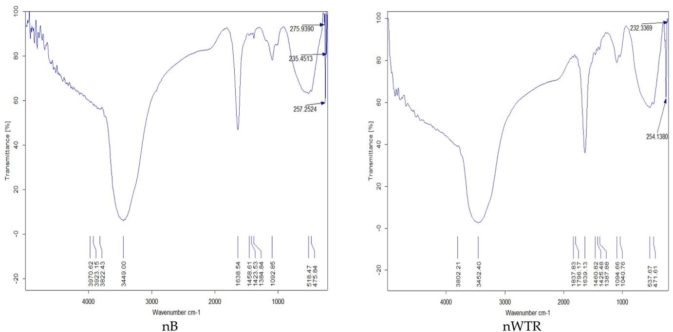
**Figure 1.** Fourier-transform infrared (FTIR) for nanobiochar (nB) and nanowater treatment residuals (nWTR).
