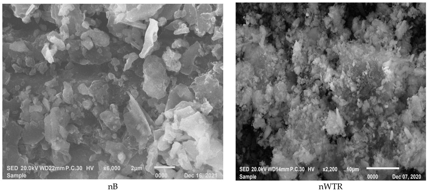
**Figure 3.** Scanning electron microscopy (SEM) images for nanobiochar (nB) and nanowater treatment re-siduals (nWTR).
