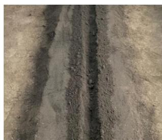
Figure 12. Soil bin experiment furrow.
