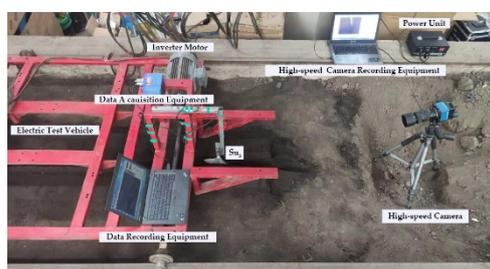
Figure 11.  $Su_3$  experiment of soil bin.
