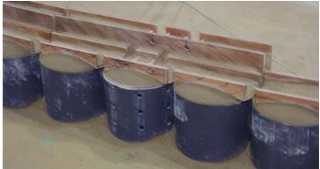
**Figure 6.** Model caissons made from UPVC pipe sections, plywood and mortar.
