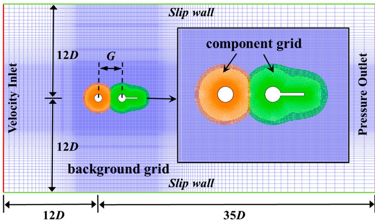
Figure 2. Grid and boundary condition settings diagram of the computing domain.
