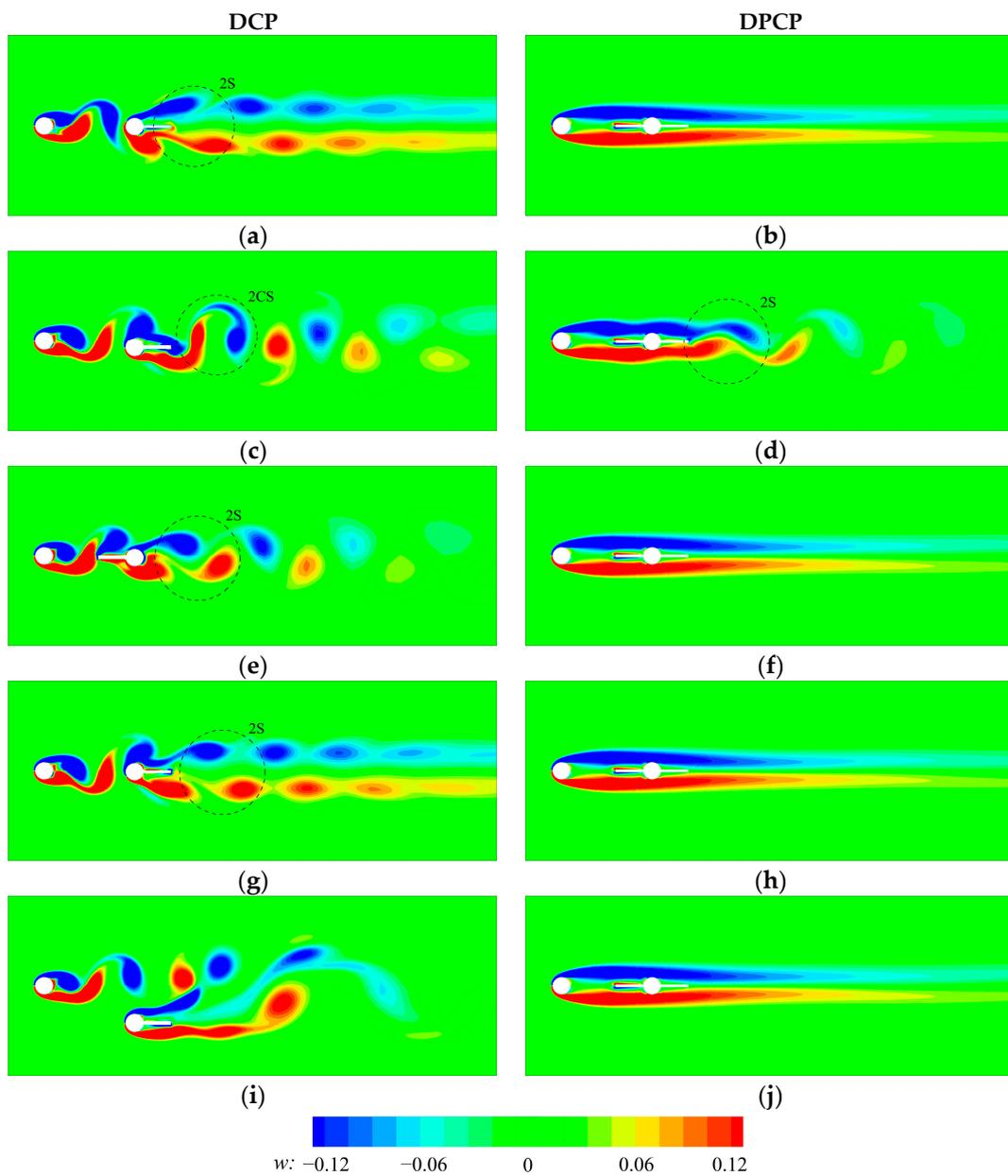
**Figure 8.** Instantaneous vorticity contours at various  $U_r$  (DCP and DPCP). (a)  $U_r = 3.0$ ; (b)  $U_r = 3.0$ ; (c)  $U_r = 5.0$ ; (d)  $U_r = 5.0$ ; (e)  $U_r = 10.0$ ; (f)  $U_r = 10.0$ ; (g)  $U_r = 15.0$ ; (h)  $U_r = 15.0$ ; (i)  $U_r = 40.0$ ; (j)  $U_r = 40.0$ .
