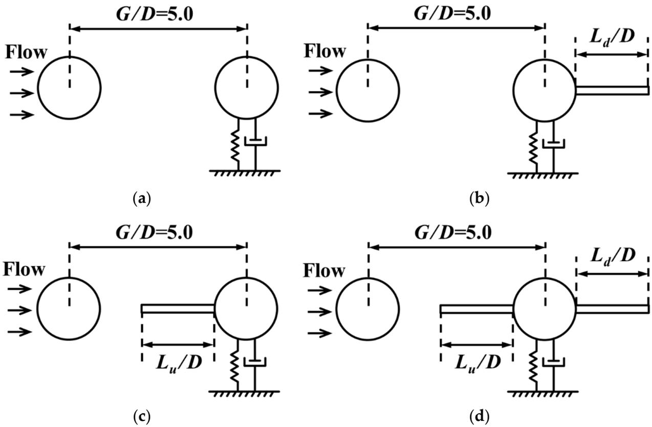
**Figure 1.** Diagram of the cylinder–plate body in different additional positions. (a) DC; (b) DCP; (c) DPC; (d) DPCP.
