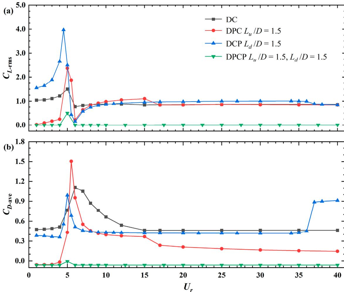
Figure 6. Variations in the  $C_{L-rms}$  and  $C_{D-ave}$  at different splitter plate additional positions against  $U_r$ .
