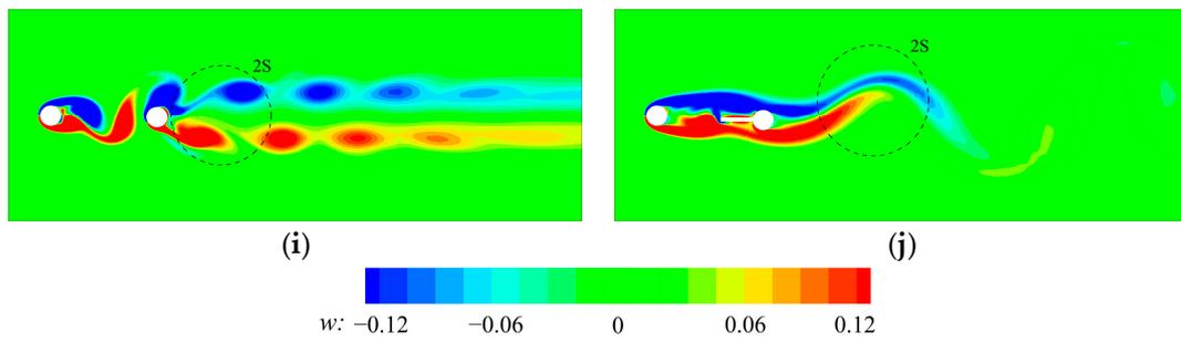
**Figure 7.** Instantaneous vorticity contours at various  $U_r$  (DC and DPC). (a)  $U_r = 3.0$ ; (b)  $U_r = 3.0$ ; (c)  $U_r = 6.0$ ; (d)  $U_r = 5.5$ ; (e)  $U_r = 10.0$ ; (f)  $U_r = 10.0$ ; (g)  $U_r = 15.0$ ; (h)  $U_r = 17.0$ ; (i)  $U_r = 40.0$ ; (j)  $U_r = 40.0$ .
