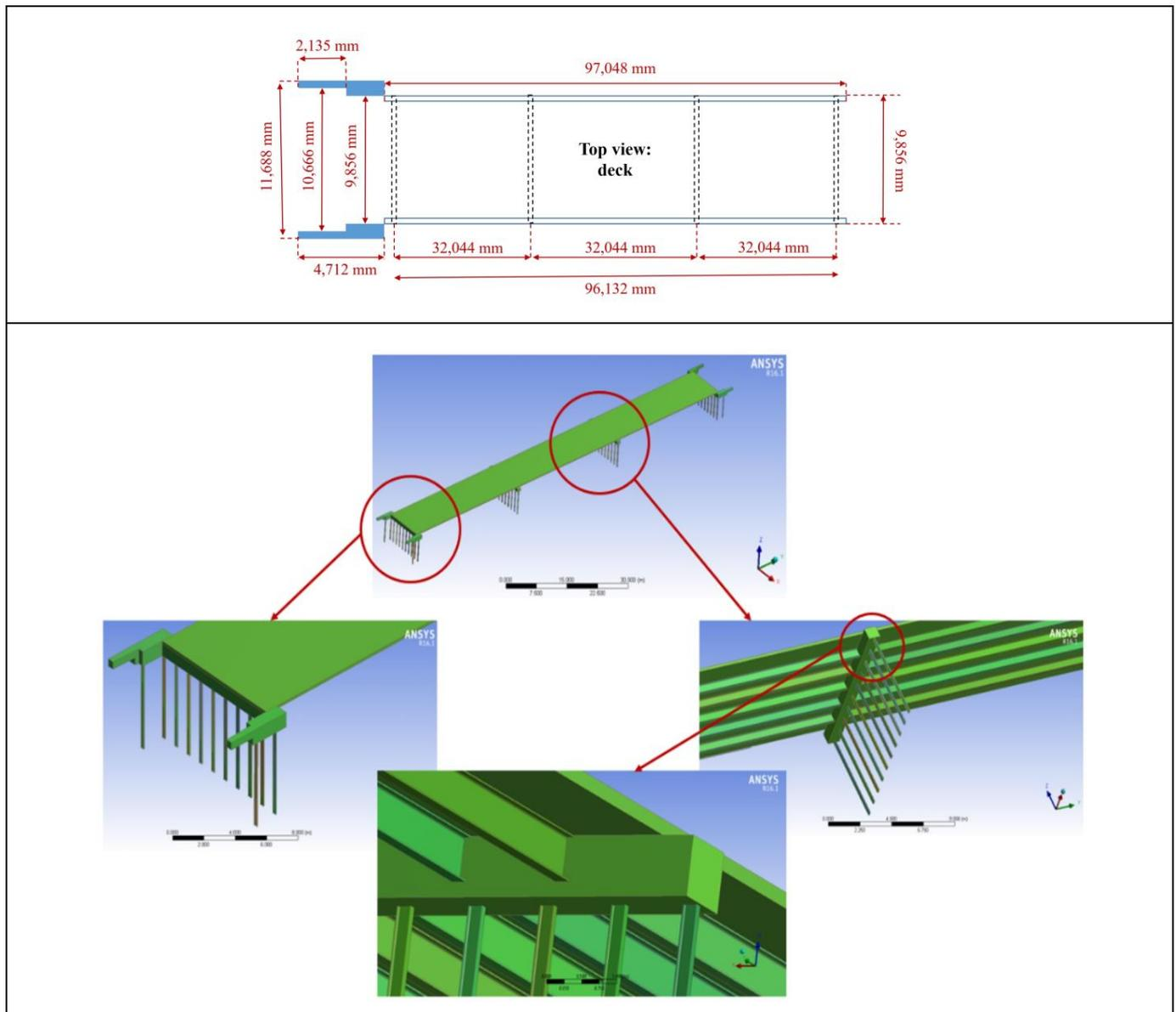
**Figure 4.** Details of the geometric model of the studied bridge in real scale [1].
