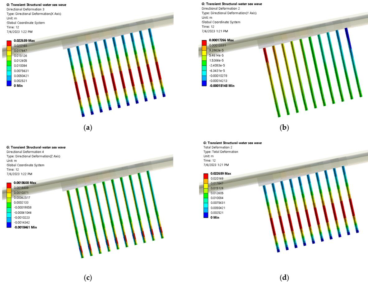
Figure 11. Deformation contours in N3 row steel piles of the bridge due to the impact of waves: (a) deformation in X direction, (b) deformation in Y direction, (c) deformation in Z direction, and (d) total deformation.
