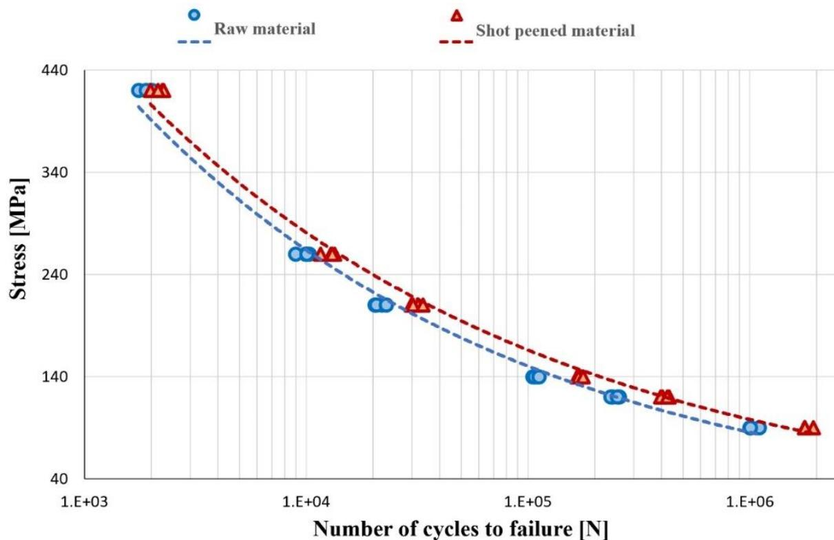
**Figure 3.** The HCF behavior of shot peened St52 compared to the raw material.
