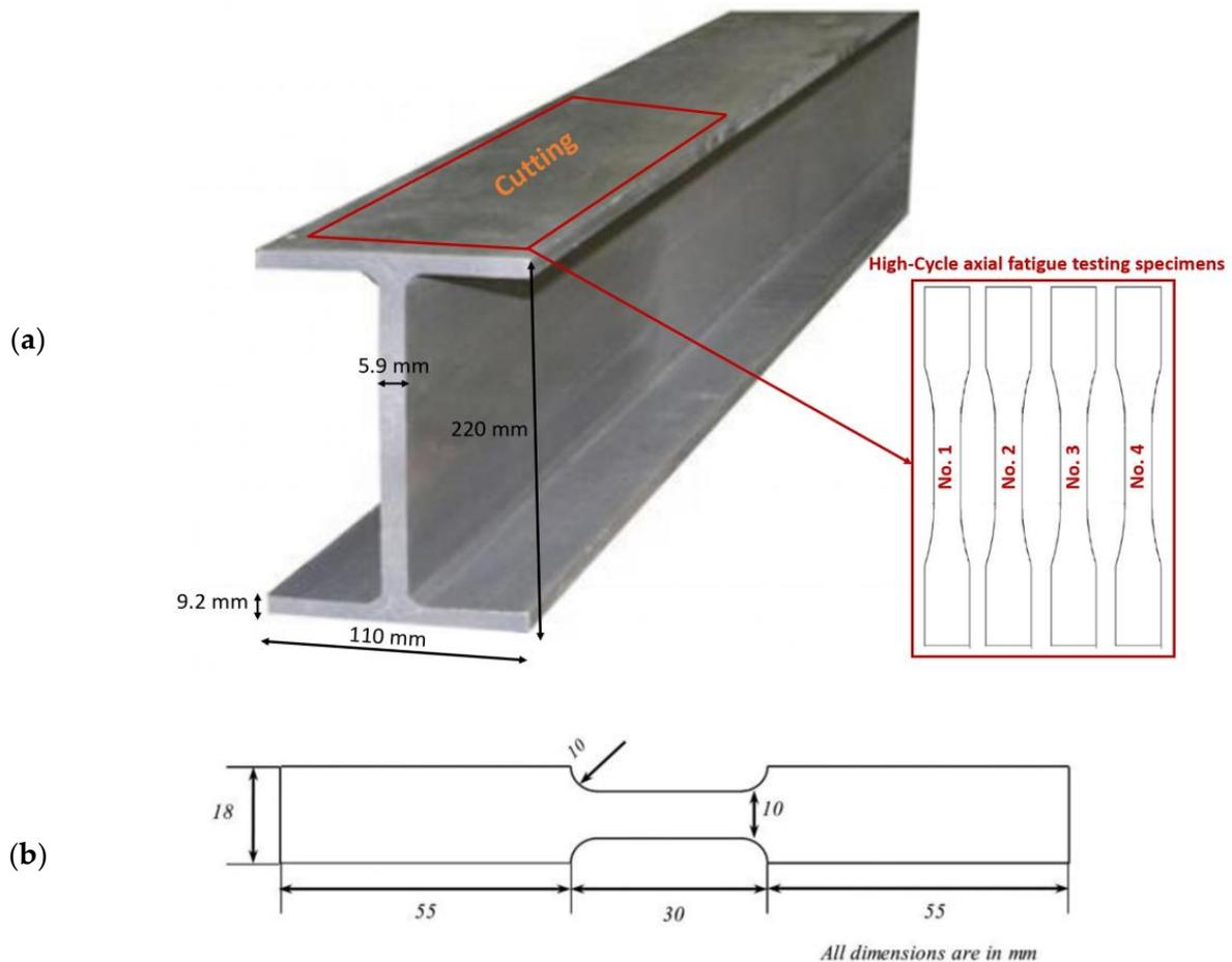
**Figure 2.** Preparation of experiment specimens: (a) exact place where the specimens were cut from the steel beam and (b) geometry and dimensions of test specimens according to the ASTM standard for conducting axial HCF test [1].
