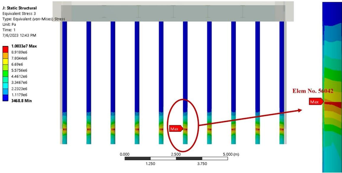
Figure 10. The exact location of the critical element prone to failure: element No. 56,042 at location of S28 in row N3.
