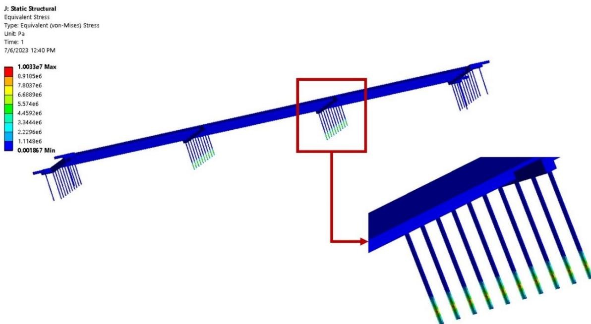
Figure 9. Von Mises equivalent stress contour in the bridge steel piles due to the pressure of motionless water and temperature difference of air (22 °C) and water (7 °C).
