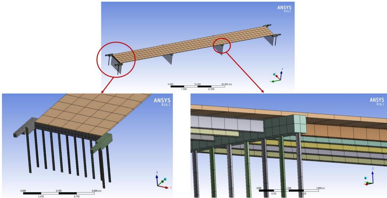
**Figure 6.** Finite element model of the bridge after mesh convergence study [16].
