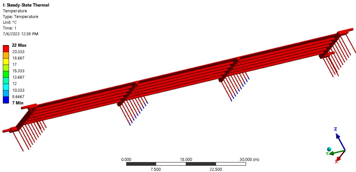
Figure 8. Temperature distribution in the bridge as a result of steady-state thermal analysis.
