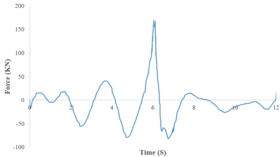
**Figure 7.** Loading history considered for the impact of sea waves with a height of 25 cm [16].
