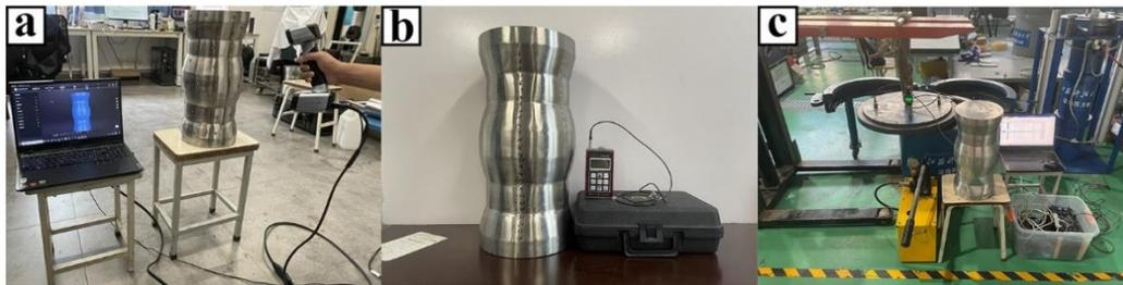
**Figure 7.** Photographs of experimental setups for the fabricated preform: (a) geometric measurement, (b) thickness measurement, and (c) hydrostatic test.
