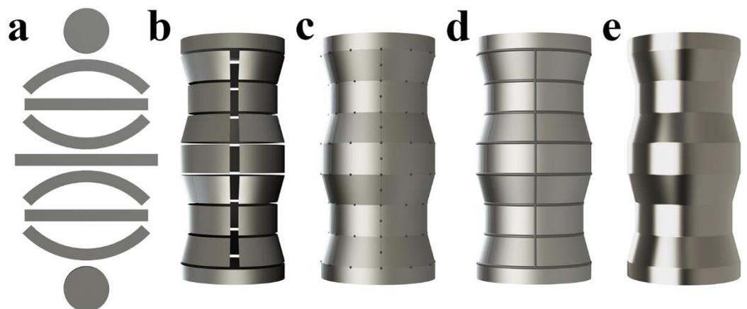
**Figure 6.** Preform fabrication involving (a) blanking, (b) bending, (c) assembly, (d) welding, and (e) grinding.
