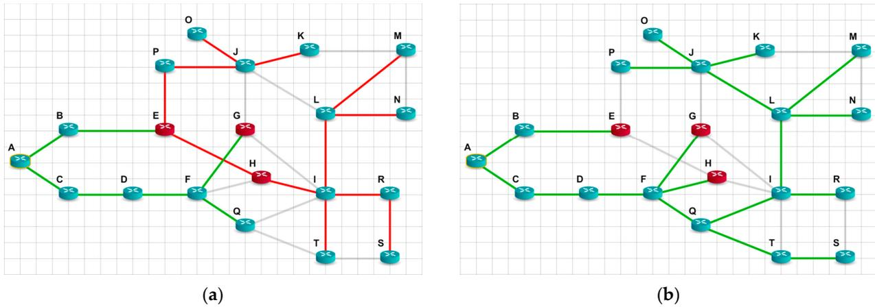
**Figure 14.** The shortest path tree for the (a) classical Dijkstra algorithm and (b) modified Dijkstra algorithm.
