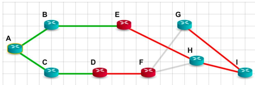
Figure 8. The shortest path tree for the network with multiple distrustful nodes, according to the modified Dijkstra algorithm.
