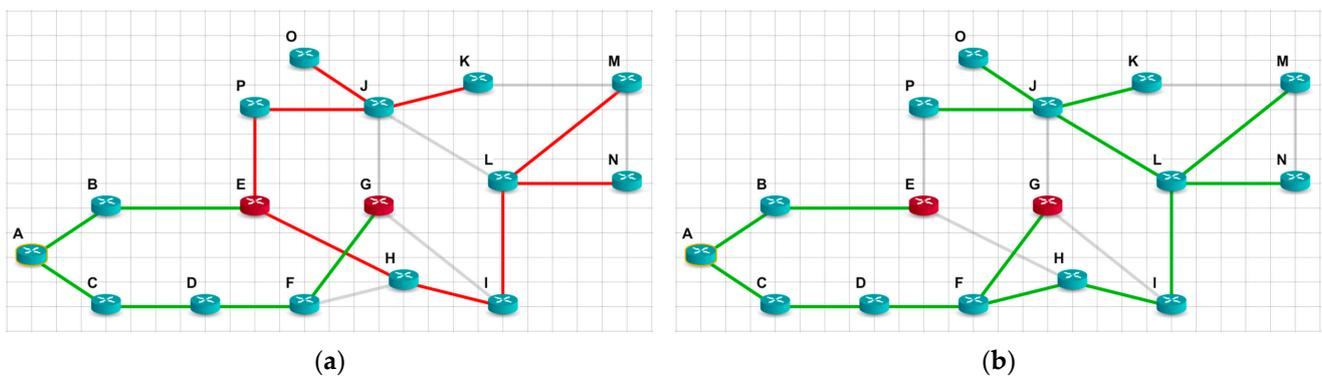
Figure 11. The shortest path tree for the (a) classical Dijkstra algorithm and (b) modified Dijkstra algorithm.
