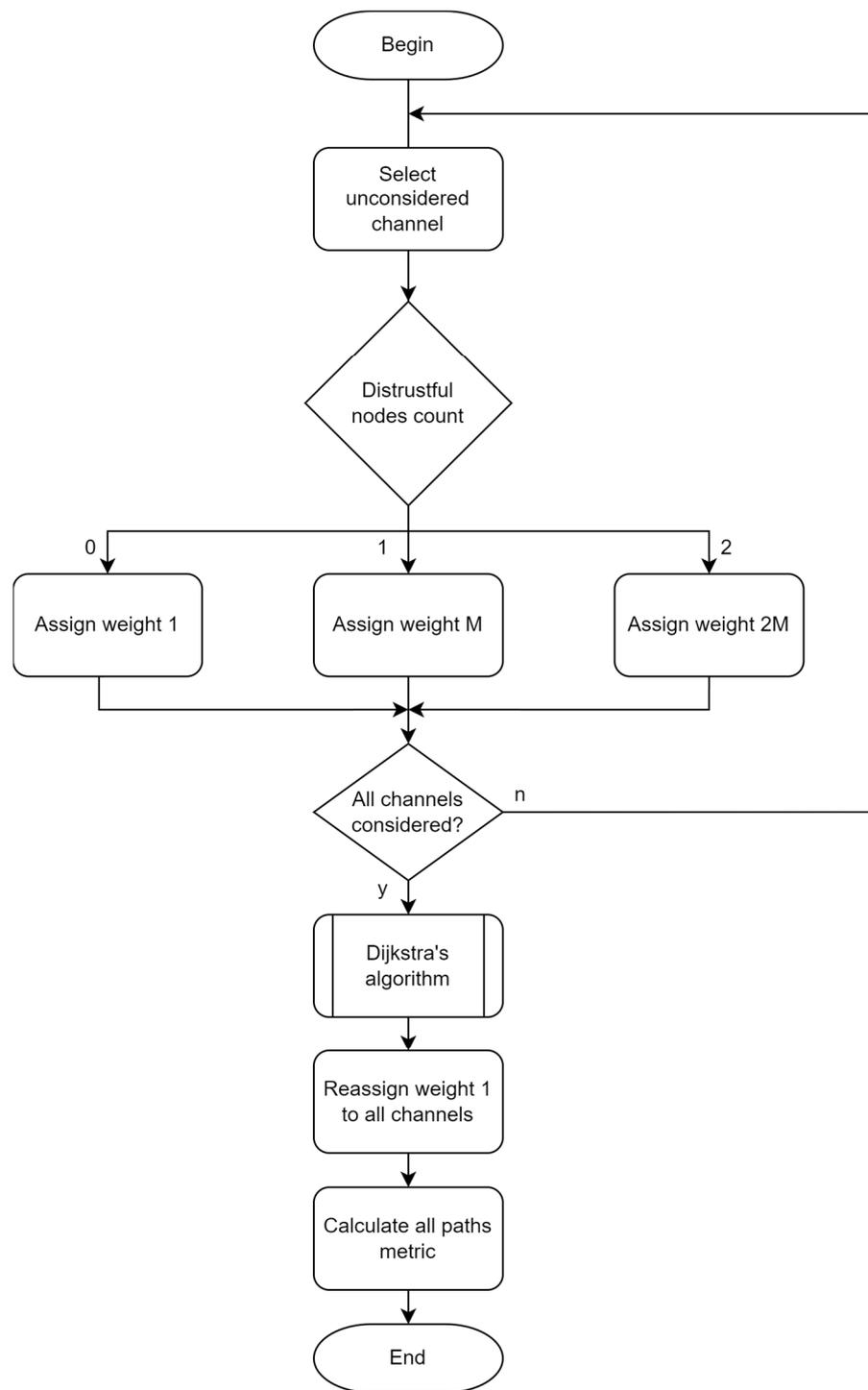
**Figure 1.** Flowchart diagram of modified algorithm.
