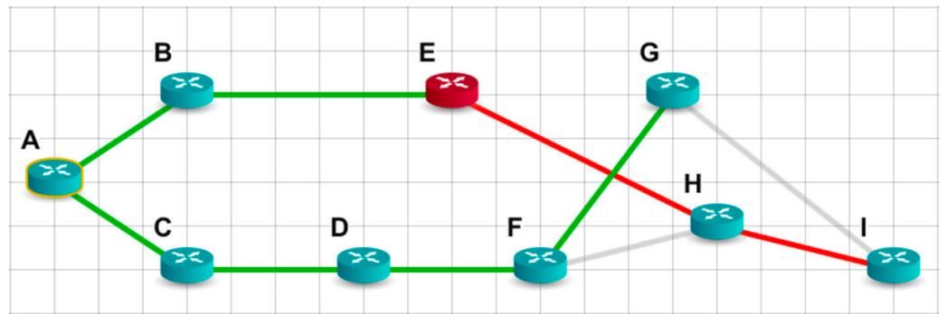
**Figure 3.** The shortest path tree for node A, according to classical Dijkstra’s algorithm.
