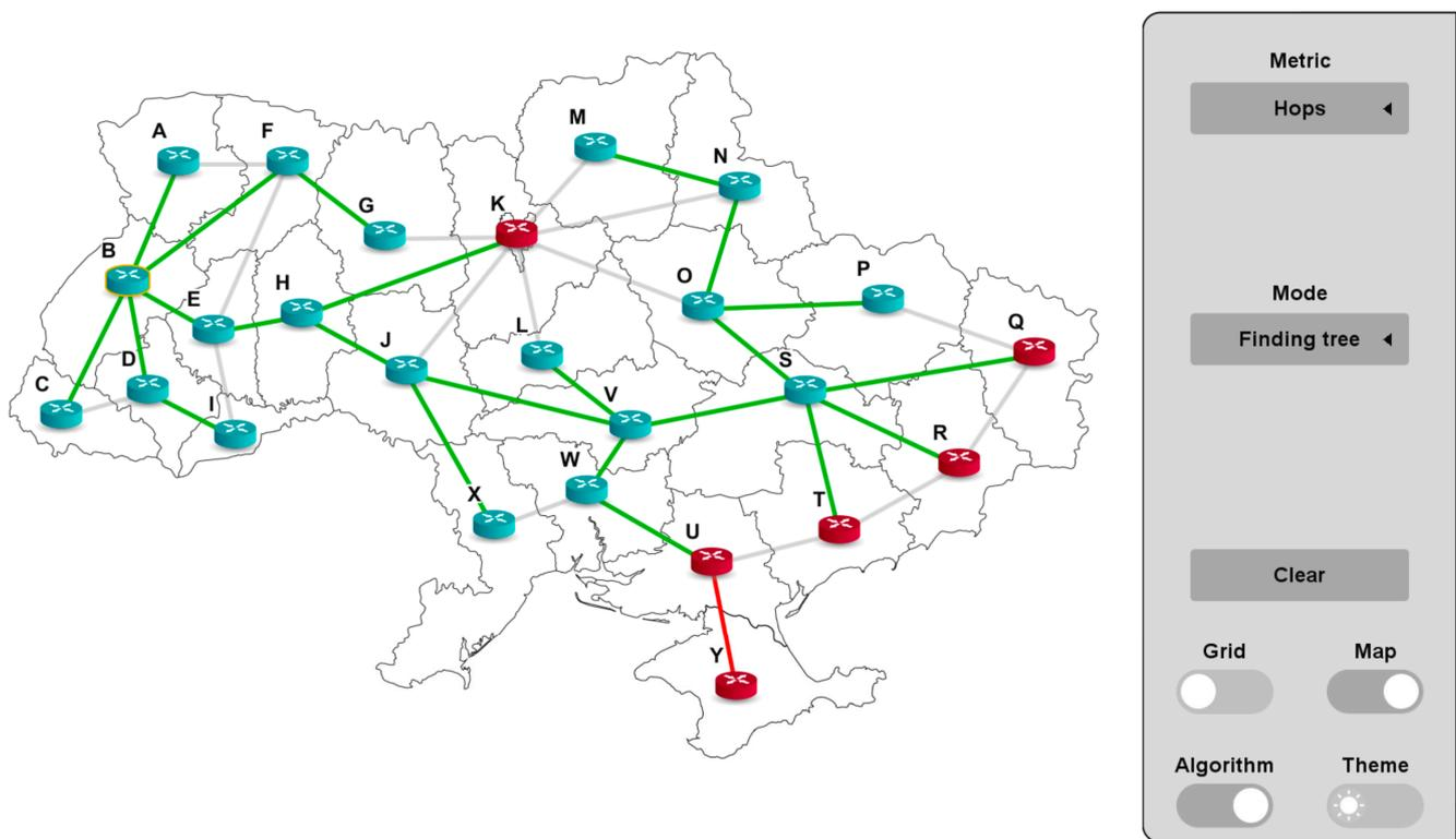
**Figure 17.** The shortest path tree, according to the modified Dijkstra algorithm.
