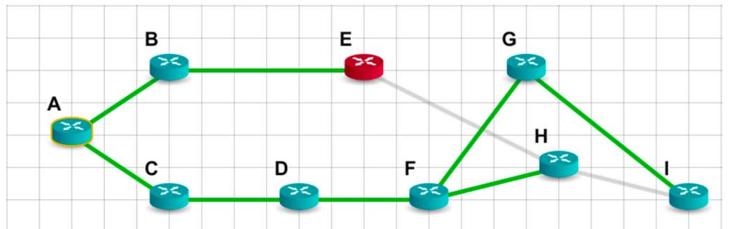
**Figure 4.** The shortest path tree for node A, according to the modified Dijkstra algorithm.
