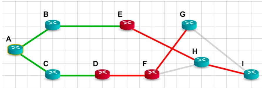
Figure 7. The shortest path tree for the network with multiple distrustful nodes, according to the classical Dijkstra algorithm.
