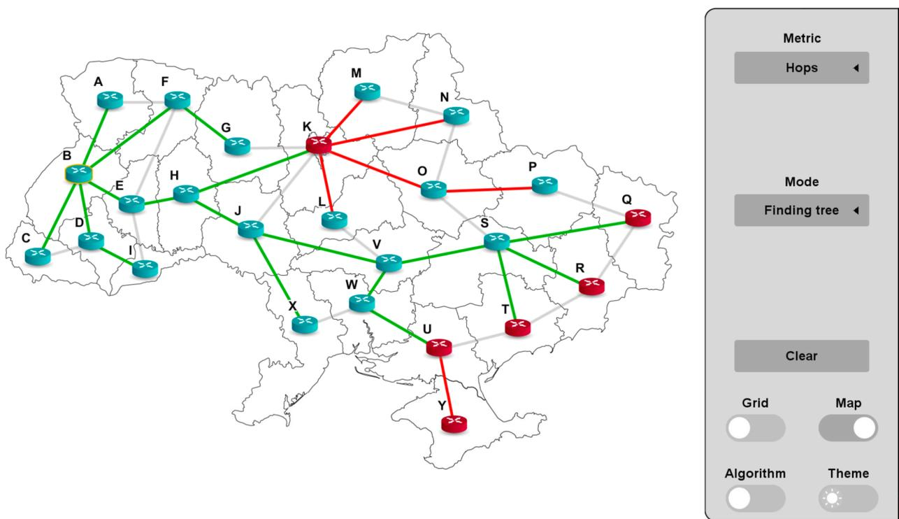
Figure 16. The shortest path tree, according to the classical Dijkstra algorithm.
