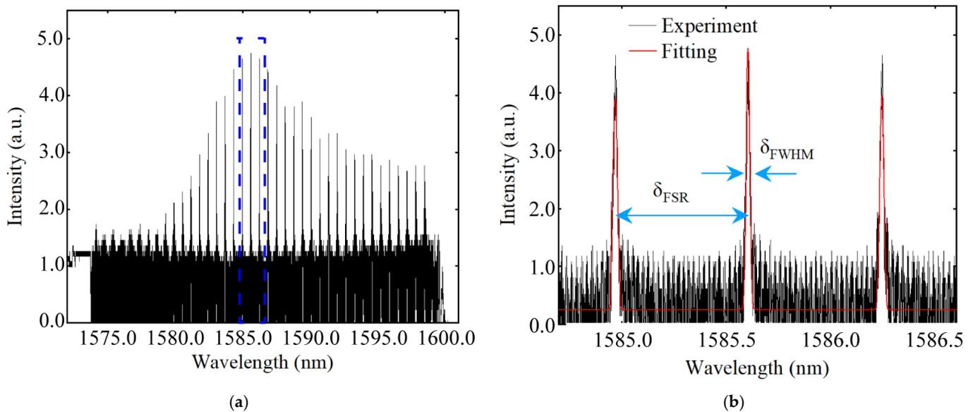
**Figure 7.** The transmission power spectrum of the F-P cavity. (a) The transmission power spectrum of the F-P cavity ranging from 1572–1601 nm when the output power of the tunable laser is 1 mW. The measured FSR is 0.647; (b) The partial transmission power spectrum and its fitted curve range from 1584.7 nm to 1586.6 nm. The measured  $f_R$  is 38 when the measured FWHM is 0.017 near 1585 nm.
