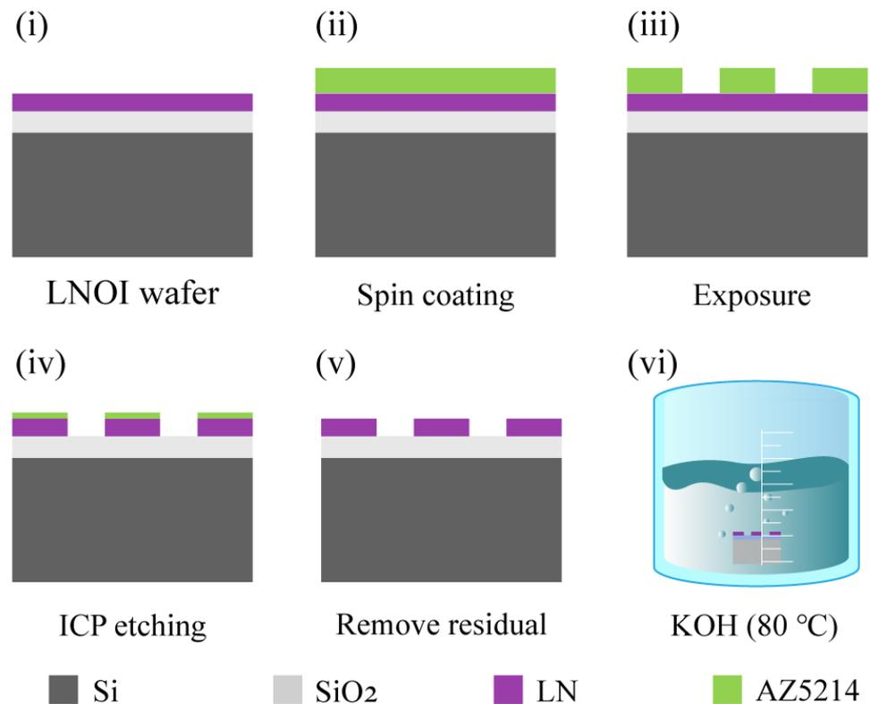
**Figure 2.** The device fabrication process. (i) The x-cut LNOI wafer; (ii): Spin-coating photoresist; (iii) Defining the pattern of the LN metasurface by Stepper lithography; (iv) Transferring the pattern of the LN metasurface onto the LN layer by inductively coupled plasma (ICP) etching; (v) Removing the residual resist; (vi) The fabricated LN metasurface was immersed in 0.5 mol/L KOH solution at 80 °C for 20 min to further improve the etching quality.
