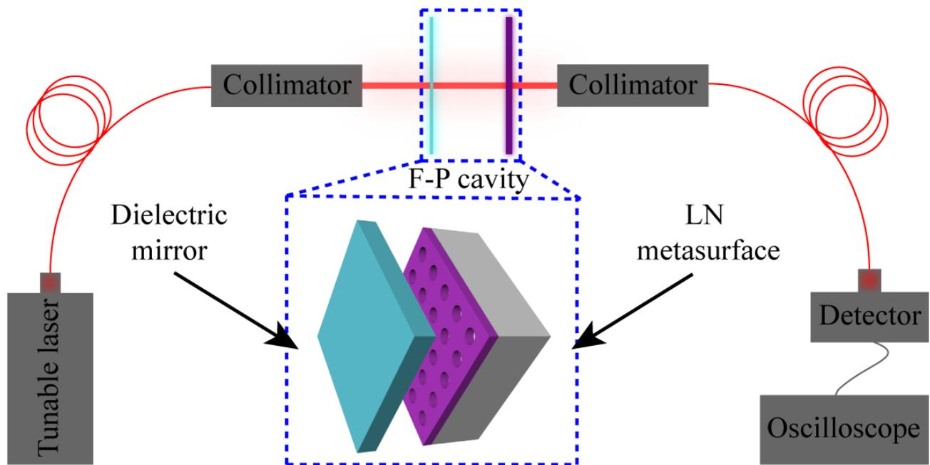
**Figure 6.** The F-P cavity and its measurement optical path. The F-P cavity is formed by the LN metasurface and another dielectric mirror with reflectivity close to 1.
