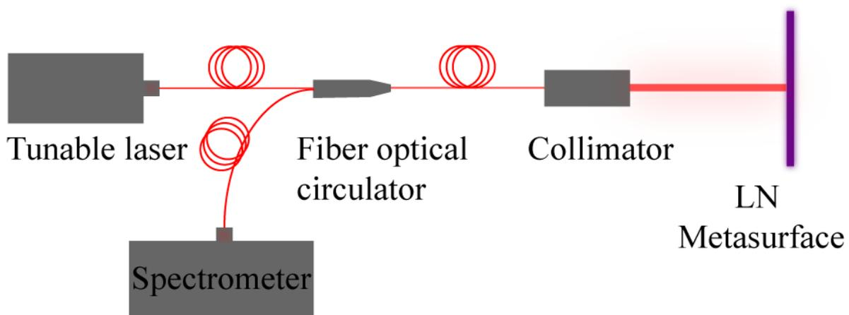
**Figure 4.** Reflectivity measurement optical path of LN metasurface.
