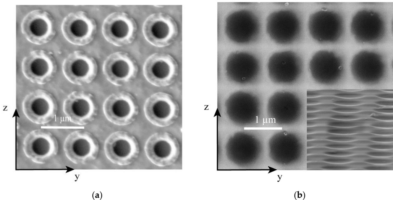
**Figure 3.** Scanning electron micrograph (SEM) images of the fabricated LN metasurfaces along the  $yz$  plane. (a) The top-view SEM image of the fabricated LN metasurface after ICP etching and before KOH wet etching; (b) The top-view SEM image of the fabricated LN metasurface after KOH wet etching; the inset is the tilt- $10^\circ$  view image.
