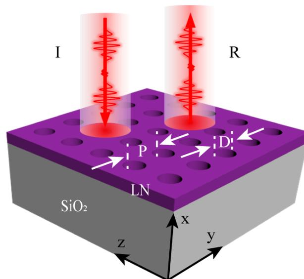
**Figure 1.** Schematic of the high-reflectivity metasurface based on  $x$ -cut LNOI comprising a square lattice of air holes, where  $P$  and  $D$  denote the period of the metasurface and the diameter of the air hole, respectively.
