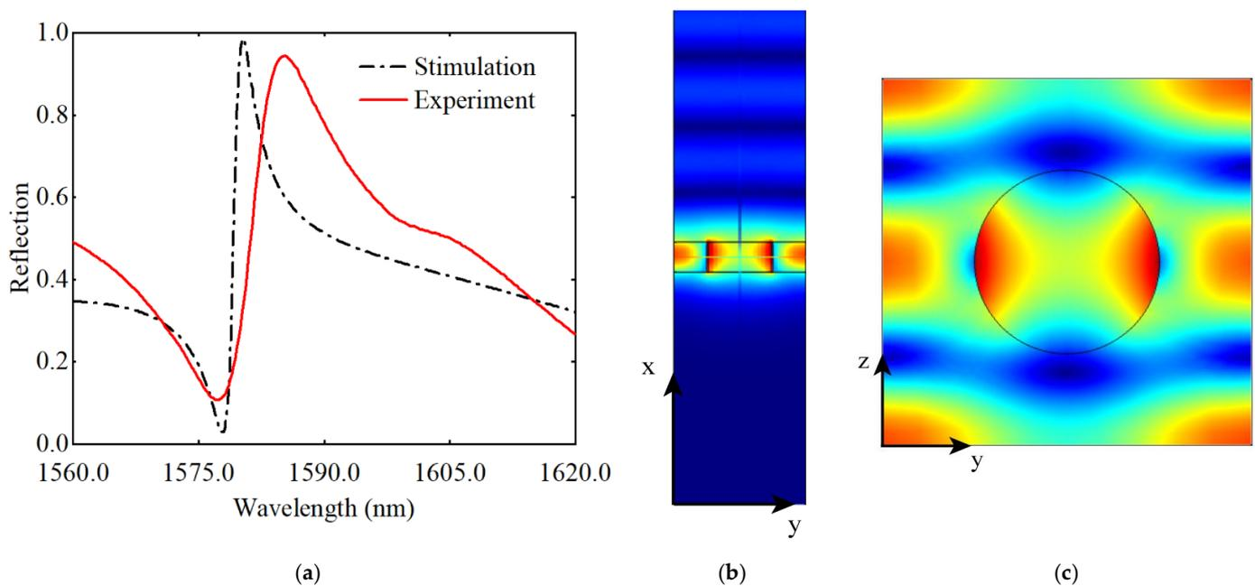
**Figure 5.** (a) The reflection of the LN metasurface in the wavelength range of 1560–1620 nm. The red line and black line are the experimental and simulated results, respectively; (b) Optical field distribution in xy plane; (c) Optical field distribution in yz plane.
