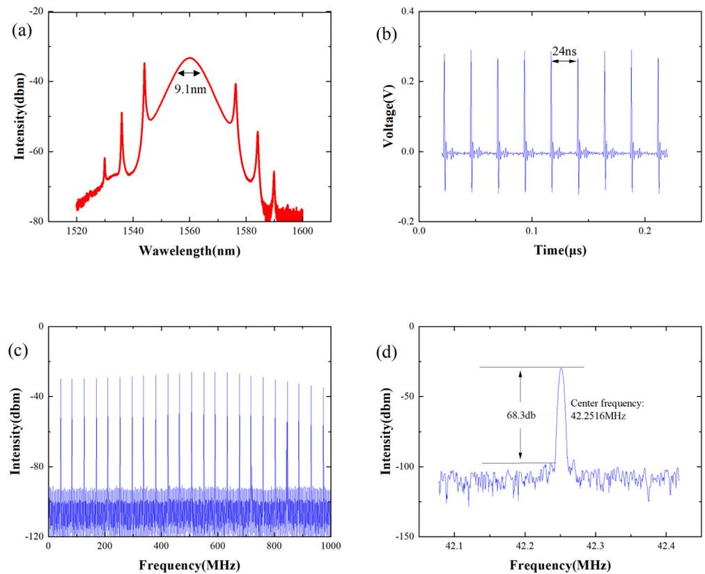
**Figure 2.** Pulse characteristics of stable soliton states. (a) Spectra; (b) pulse sequence; (c) spectrum sequence; (d) fundamental frequency signal.
