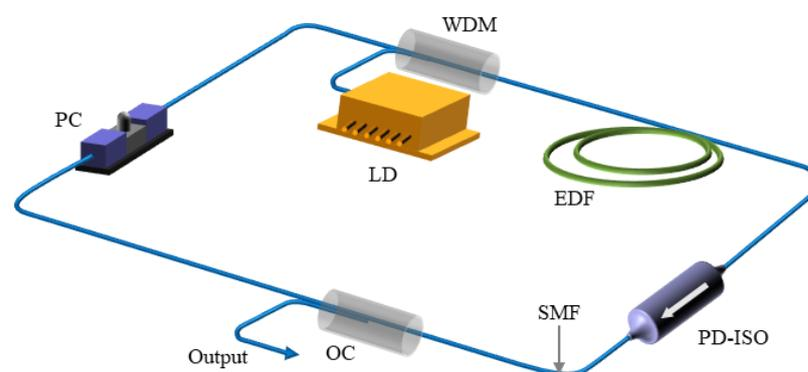
**Figure 1.** Schematic diagram of experimental setup. WDM: wavelength division multiplexer; OC: output coupler; EDF: erbium-doped fiber; PC: polarization controller; PD-ISO: polarization-related isolator.
