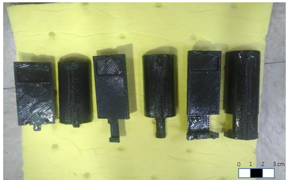
Figure 2. Micro-sensor housing after soaking.
