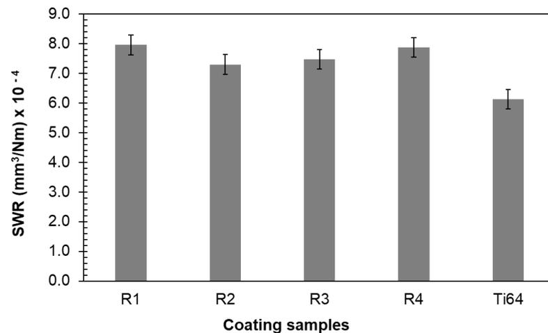
**Figure 10.** The specific wear rate of coating samples and the bulk Ti64.
