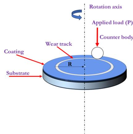
**Figure 2.** Ball-on-disk sliding wear configuration adapted from [20].
