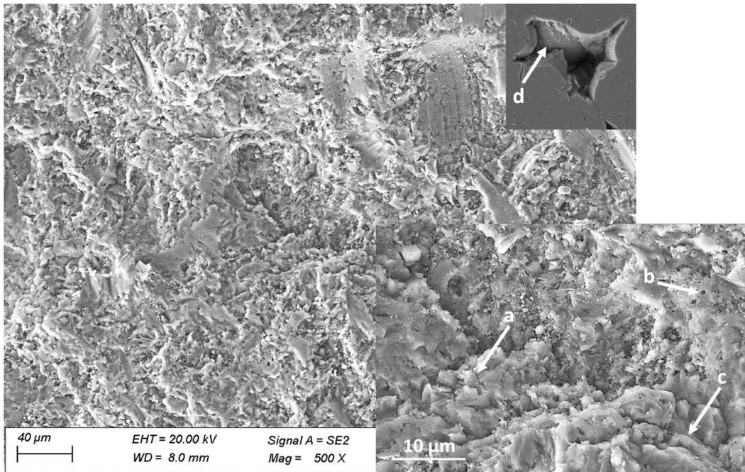
**Figure 8.** Secondary electron micrograph of the top surface morphology of the as-sprayed coatings showing (a) micro-crack, (b) blind pore, (c) inter-particle boundary, and (d) buried feedstock particle.
