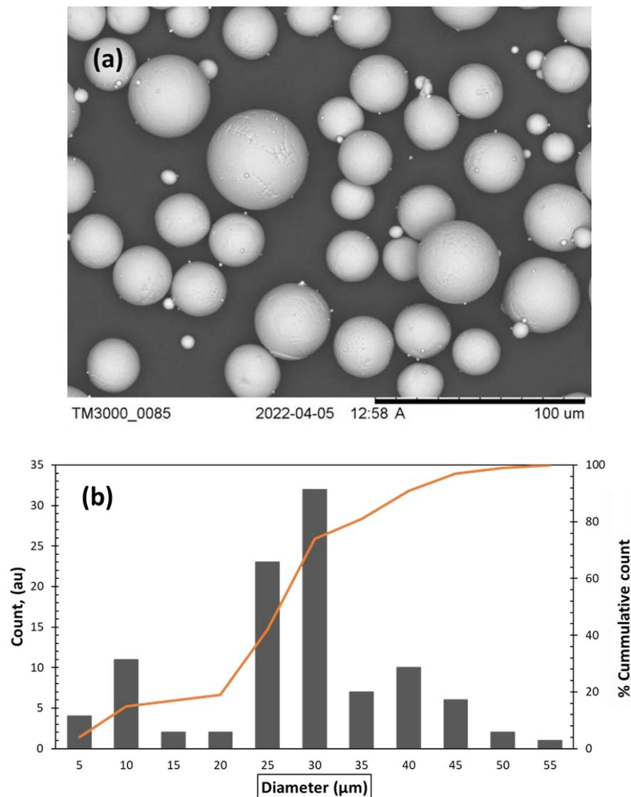
**Figure 4.** Ti64 powder feedstock. (a) Secondary electron micrograph. (b) Particle size distribution plot.
