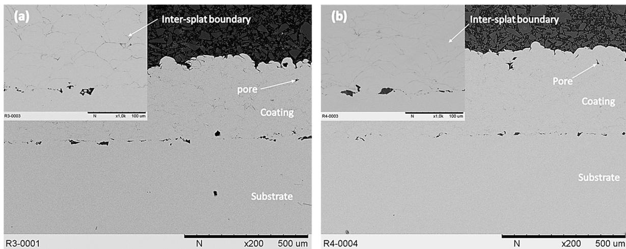
**Figure 7.** BSE micrograph of the cross-sectional images of the coatings deposited with the short nozzle. (a) Wide exit, run-3. (b) Small exit, run-4.
