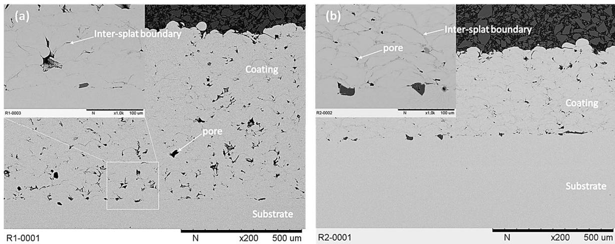
**Figure 6.** BSE micrograph of the cross-sectional images of the coatings deposited with the long nozzle. (a) Wide exit, run-1. (b) Small exit, run-2.
