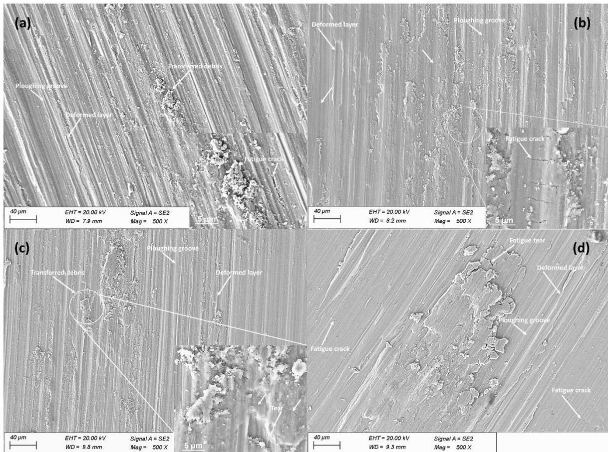
**Figure 11.** Secondary electron micrograph of wear tracks generated on the surfaces of (a) run-1, (b) run-2, (c) run-3, and (d) run-4, showing grooves, transferred materials, fatigue cracks, and deformed layers.
