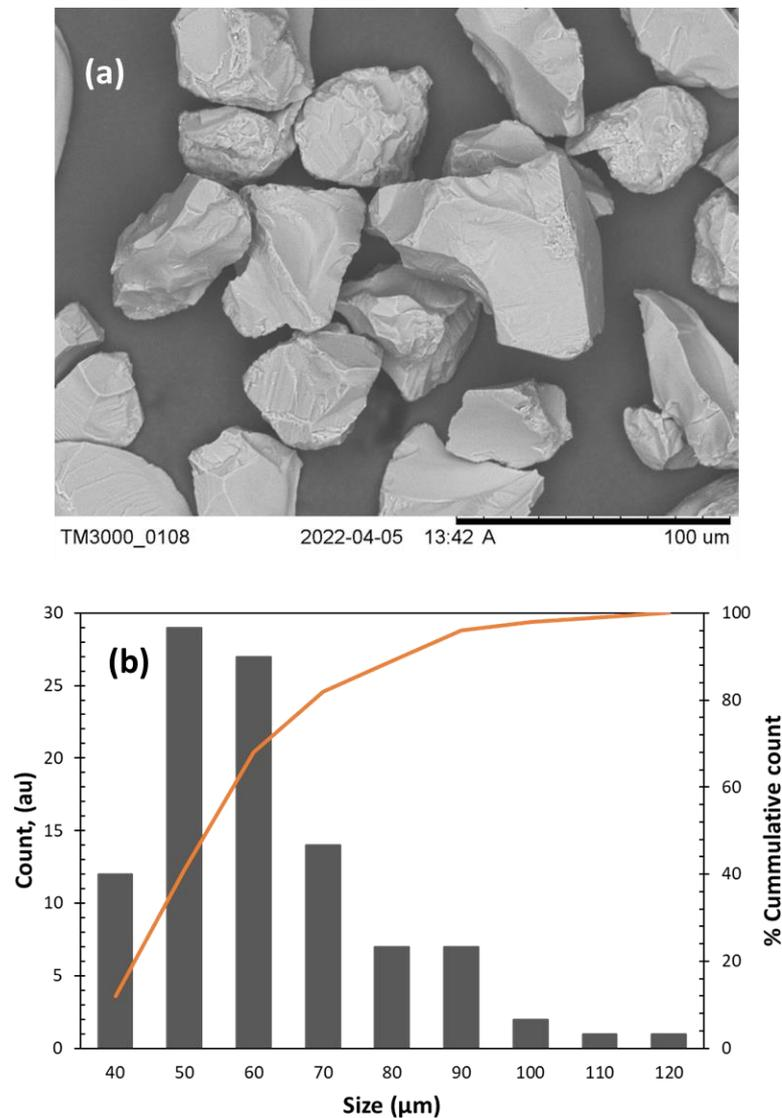
**Figure 5.** Al<sub>2</sub>O<sub>3</sub> erodent powder feedstock. (a) Secondary electron micrograph. (b) Particle size distribution plot.
