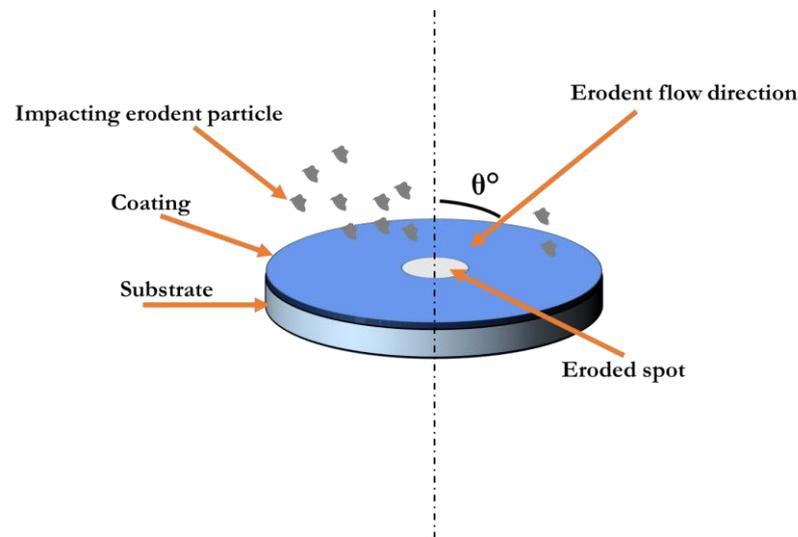
**Figure 3.** Schematic showing the erosion test configuration adapted from [21].
