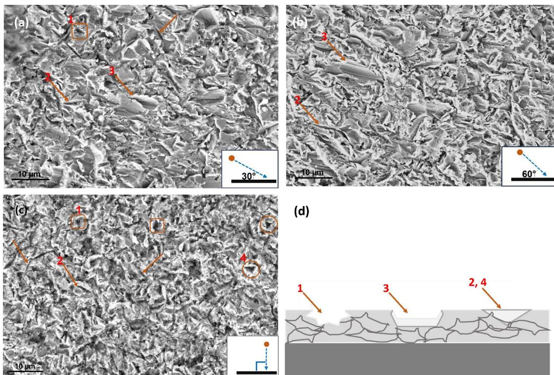
**Figure 14.** Representative magnified SE micrographs showing residual imprints eroded surfaces at angles of (a)  $30^\circ$ , (b)  $60^\circ$ , and (c)  $90^\circ$  and a (d) schematic representation of the dominant mechanisms across the three surfaces.
