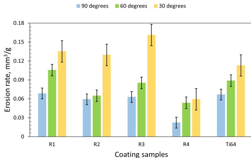
**Figure 12.** The erosion wear rate of coating samples and the bulk Ti64 sample.
