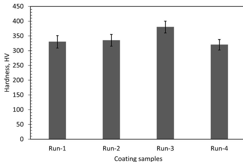
**Figure 9.** Vickers hardness value for four coating samples.
