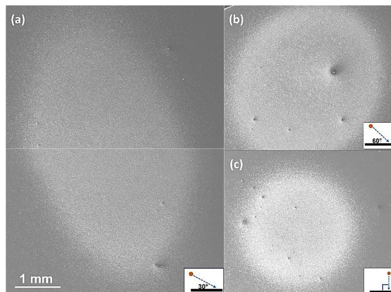
**Figure 13.** Representative SE micrograph showing overviews of erodent impacted sites per incident angle of the erodent to the sample surface: (a) 30°, (b) 60°, and (c) 90°.
