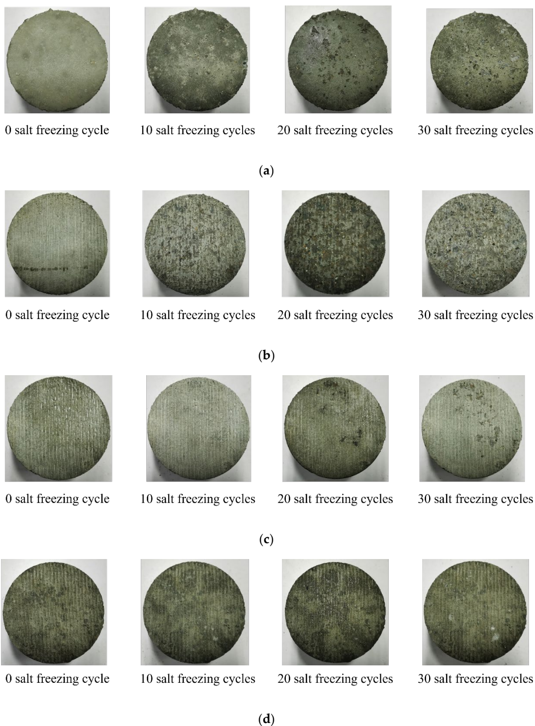
Figure 11. (a) Smoothing; (b) brushing; (c) brushing + spraying silane; and (d) brushing + silane-impregnated.
