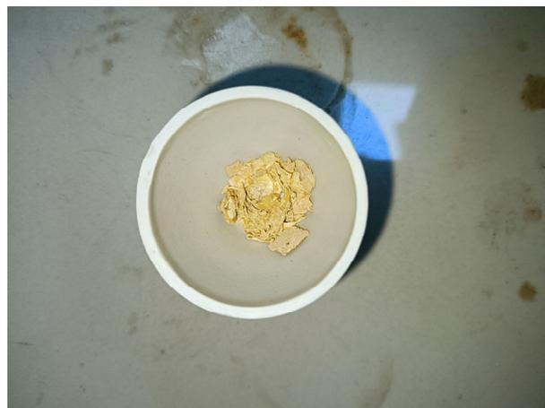
**Figure 6.** Photo of Ti60 matrix oxidized at  $1100 \text{ }^\circ\text{C} \times 60 \text{ h}$ .
