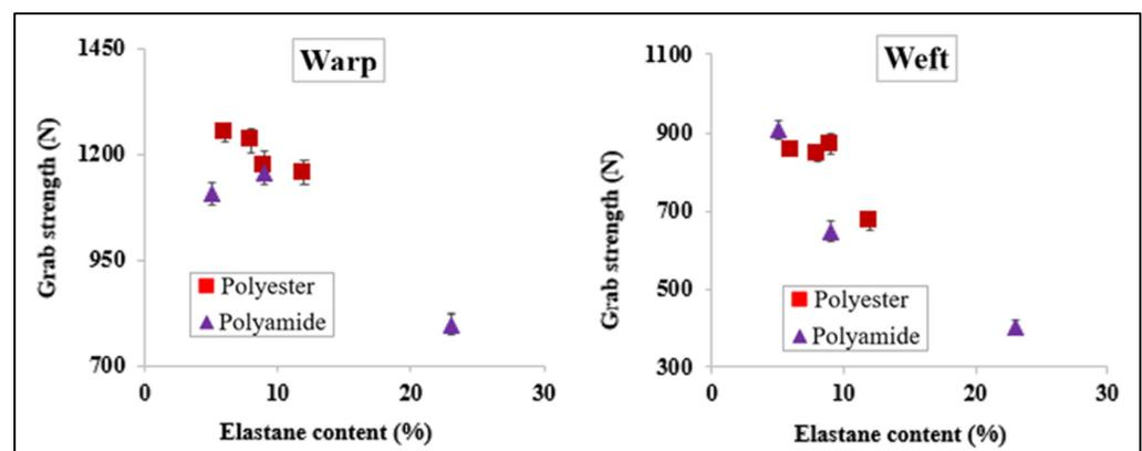
Figure 7. Variation of the fabric grab strength as a function of the elastane content in both directions.
