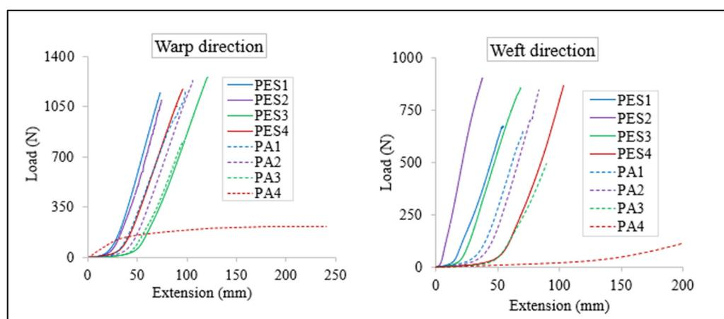
**Figure 2.** Load–extension curves of the fabrics under study in the warp and weft directions.
