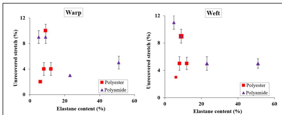
**Figure 11.** Variation of the fabric unrecovered stretch as a function of the elastane content in both directions.
