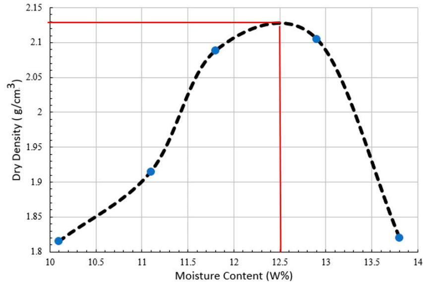
Figure 3. Proctor compaction results for soil mix with 5% cement (weight of cement to soil).
