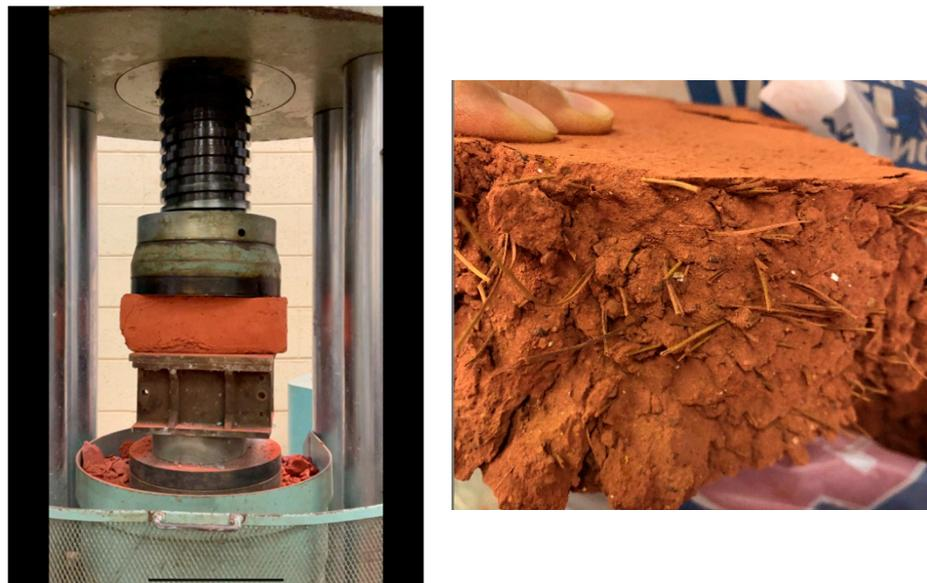
Figure 5. Mudbricks during and after loading.
