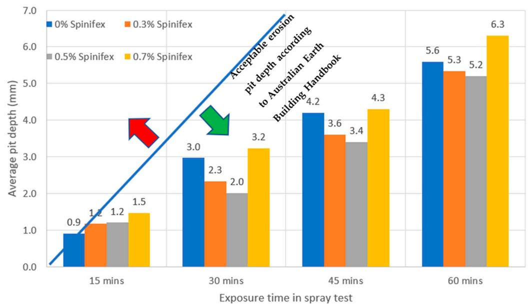
**Figure 9.** Average values of pit depth in accelerated erosion test.
