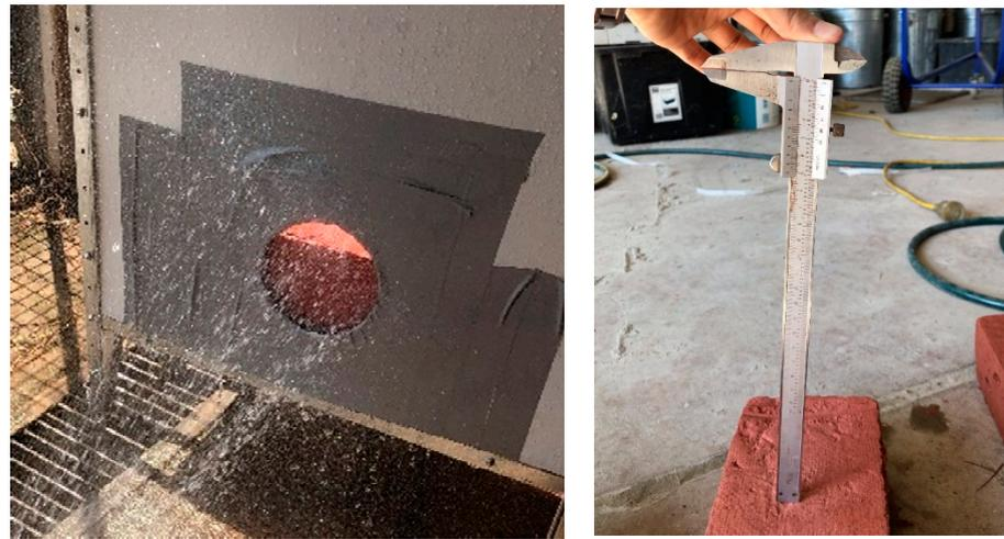
**Figure 8.** Left: test setup for accelerated erosion test. Right: measuring the pit depth using vernier callipers.
