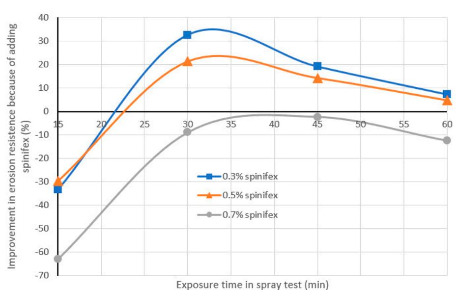
**Figure 10.** Effectiveness of spinifex inclusion in improving erosion resistance.
