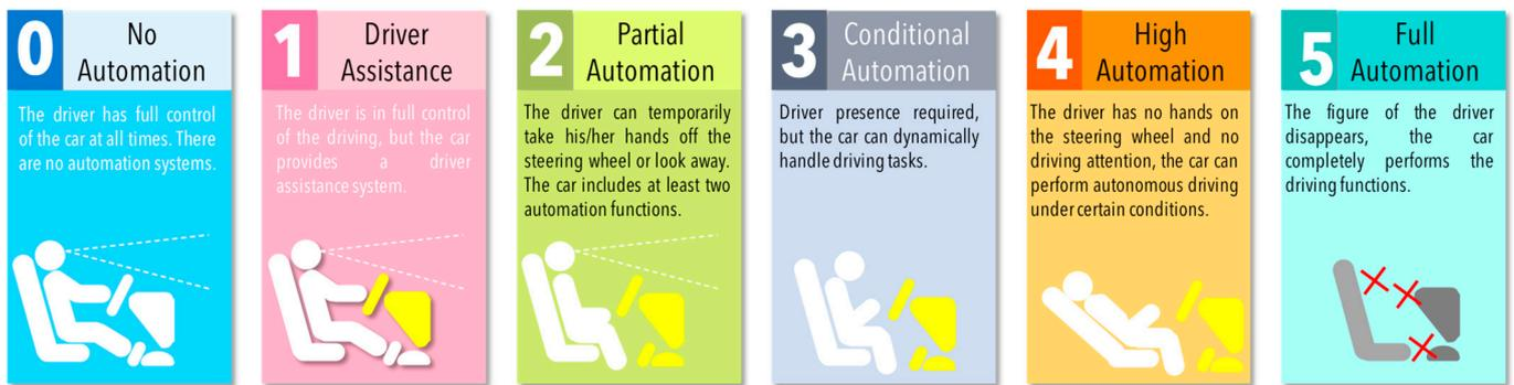
**Figure 1.** Levels of vehicle driving automation defined by the Society of Automotive Engineers.
