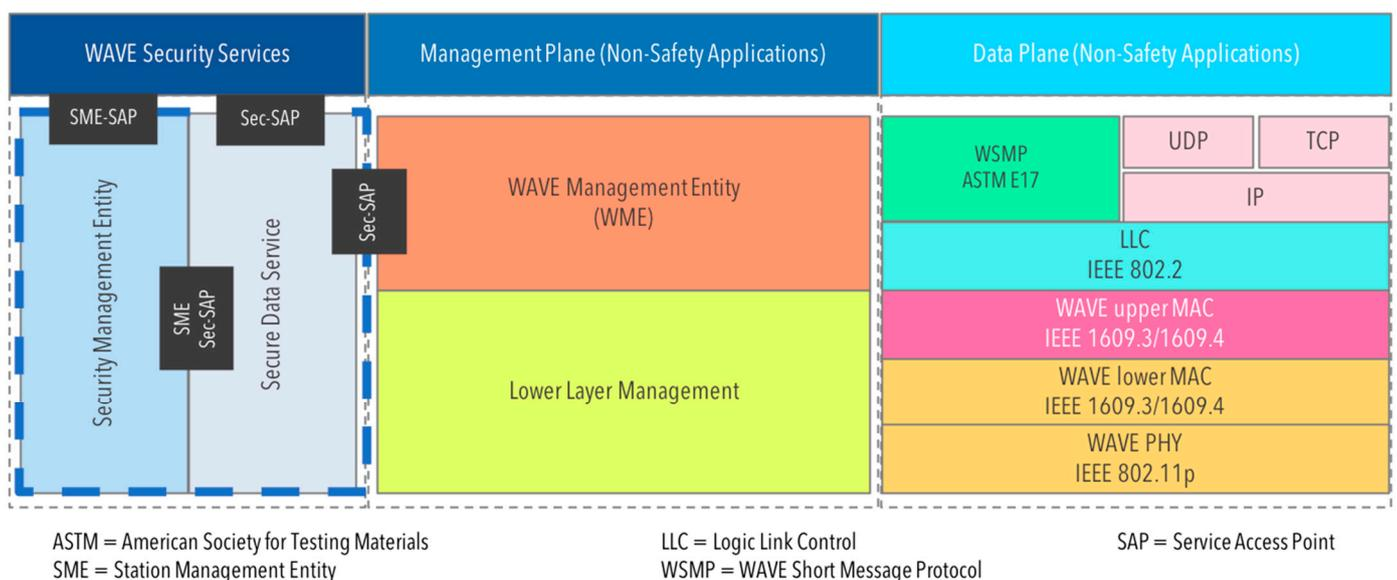
Figure 3. Representation of the WAVE reference model.
