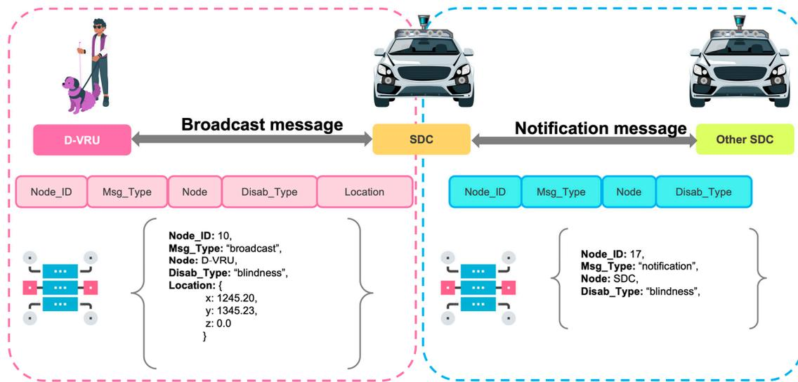
Figure 6. Representation of the type of messages defined for data exchange.
