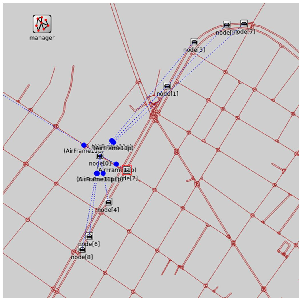
**Figure 8.** Representation of the simulation scenario in Veins. The overlapped messages represent IEEE 802.11p broadcasting frames sent by the D-VRU to neighboring vehicles.
