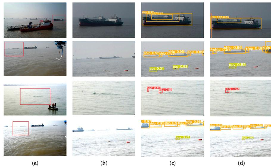
**Figure 7.** Visualization of the detection results; (a) the original image; (b) the locally enlarged image; the corresponding local enlarging is marked by red boxes in the original image in (a); (c) the detection result of the original YOLOv5 algorithm; (d) the detection result of the proposed algorithm.
