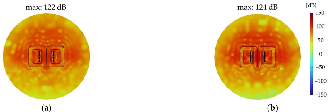
**Figure 17.** Sound pressure level distribution diagram under end-winding short circuit (a) Interleaved winding; (b) Continuous winding.
