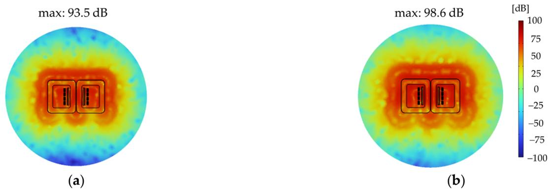
**Figure 15.** Sound pressure level distribution diagram under normal condition (a) Interleaved winding; (b) Continuous winding.
