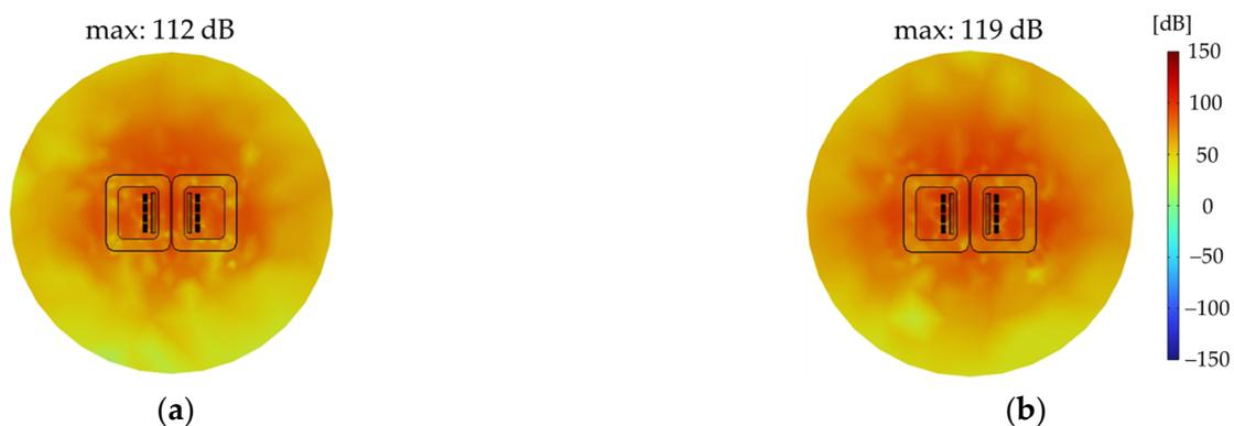
**Figure 16.** Sound pressure level distribution diagram under middle-winding short circuit (a) Interleaved winding; (b) Continuous winding.
