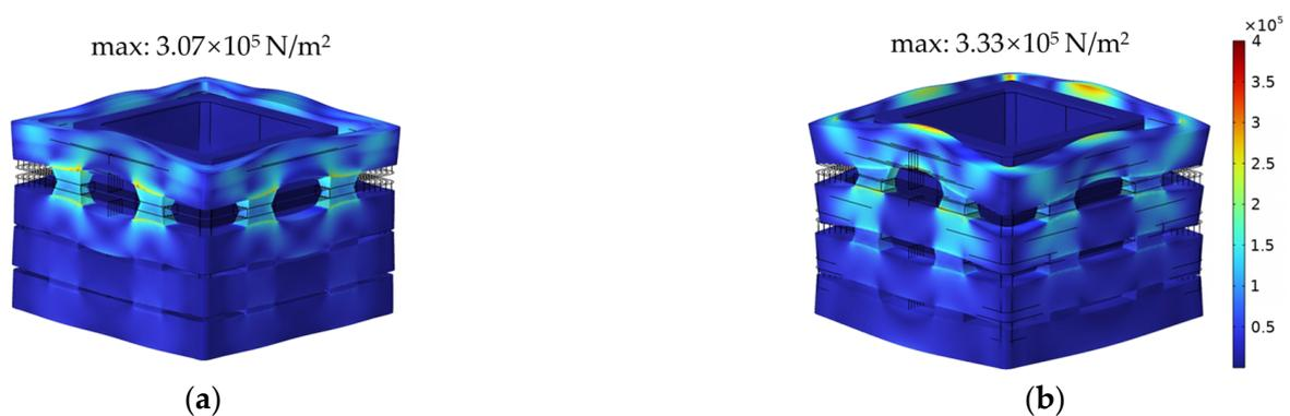
**Figure 14.** Stress distribution under end-winding short circuit (a) Interleaved winding; (b) Continuous winding.
