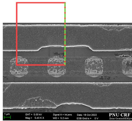
**Figure 7.** FE-SEM image of the deteriorated cells in DUTs HR-TEM was measured along a red and green dotted line.
