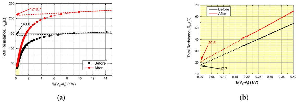
**Figure 10.**  $R_{tot}$  vs.  $(V_g - V_t)^{-1}$  graph. The y-intercept for each graph indicates the total resistance when (a)  $V_g \approx V_t$  and (b)  $V_g \gg V_t$ . The yellow region in (a) is magnified into (b).
