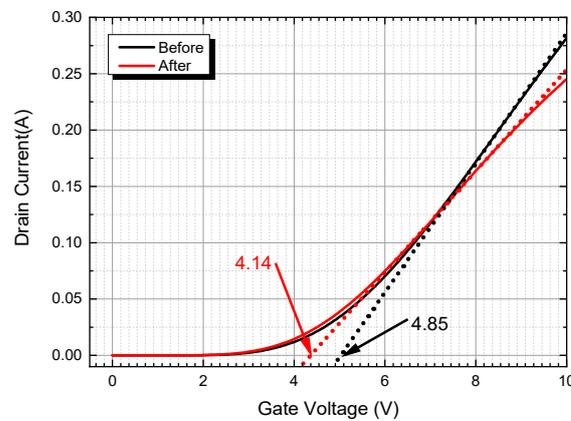
**Figure 11.** The transfer curves at a fixed, small drain voltage ( $V_d = 50$  mV). The x-intercepts is the threshold voltage before/after power cycling test.
