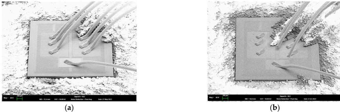
**Figure 6.** Partially decapsulated DUT images of (a) an intrinsic device and (b) a power-cycled device, whose  $V_{on}$  was increased to 120%.
