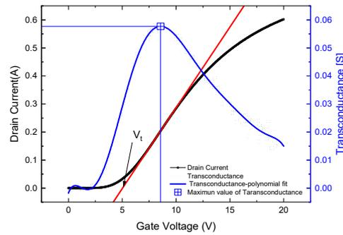
**Figure 3.** Transfer curve and transconductance of commercial high-voltage vertically double implanted 4H-SiC n-MOSFETs (VD-MOSFETs). The linear extrapolation method is applied to extract  $V_t$ .
