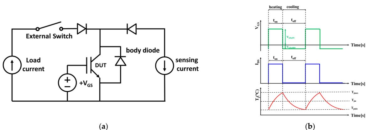
**Figure 2.** Power cycling test conditions: (a) equivalent circuit; (b) waveforms for power cycling test parameters and output junction temperature swing.
