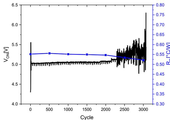
**Figure 5.** On-state voltage drop at every cycle and thermal resistance at every 500th power cycle.
