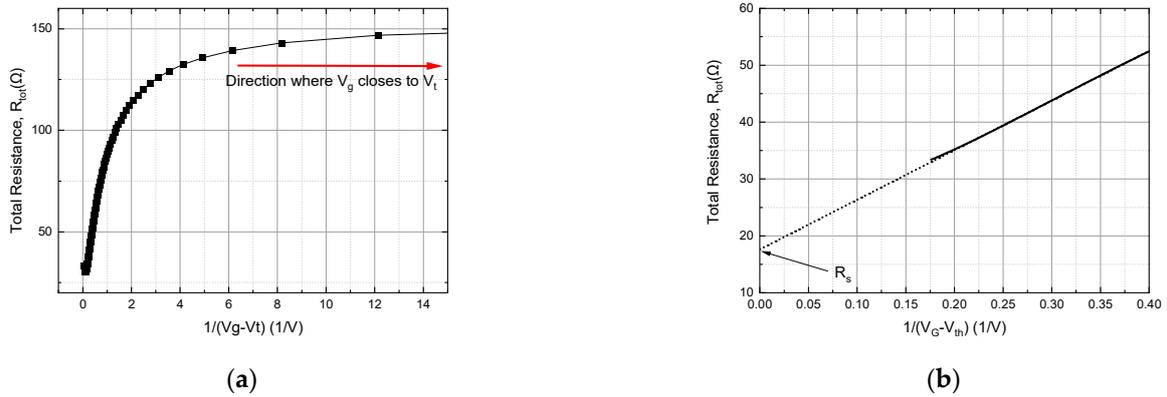
**Figure 4.**  $R_{tot}$  vs.  $(V_g - V_t)^{-1}$  graph when (a)  $V_G \rightarrow V_{TH}$ ,  $R_{CH}$  is the dominant component of  $R_{tot}$  and (b)  $\frac{1}{V_G - V_{TH}} \rightarrow 0$ . The  $y$ -intercept represents the residual resistance  $R_S$ .
