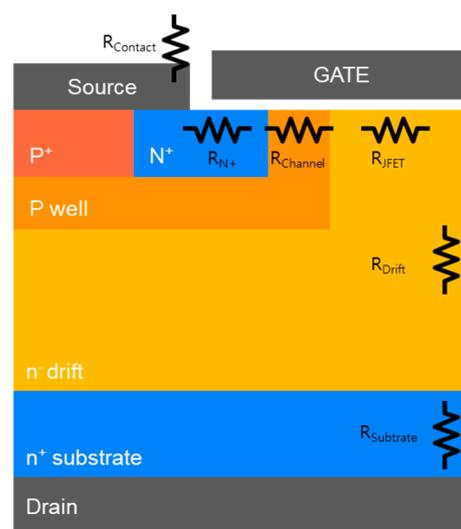
**Figure 1.** Series resistors of the total resistance ( $R_{tot}$ ).
