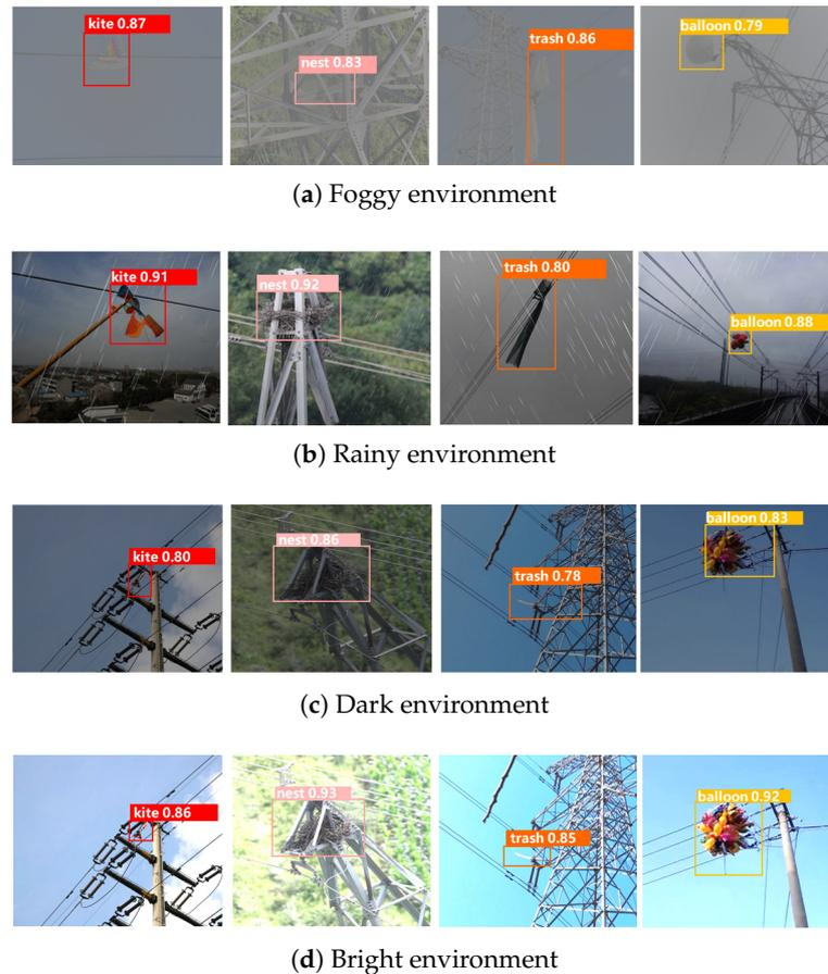
**Figure 12.** Visualisation of detection results under varying environmental conditions using the TL-YOLO algorithm. The TL-YOLO algorithm has consistent detection performance in a variety of working environments with weather conditions and lighting conditions.
