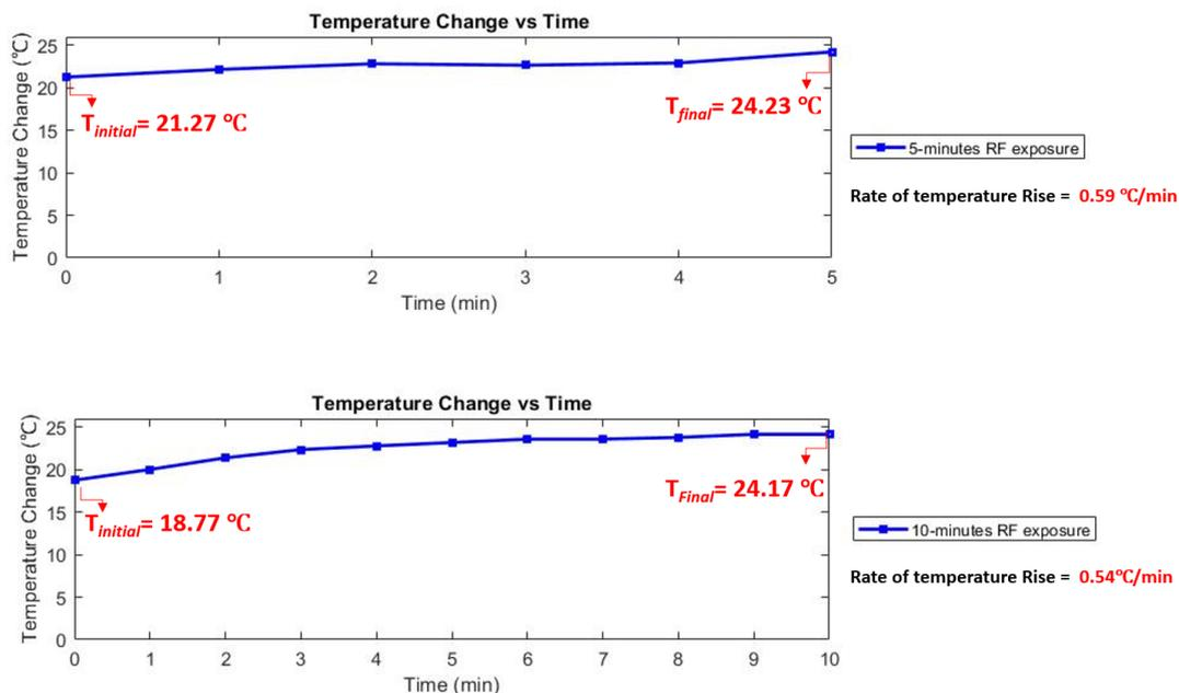
**Figure 3.** The temperature response of porcine skin to RF exposure at 26 GHz. The top image illustrates temperature variation after 5 min of exposure, while the bottom image illustrates the variation after 10 min of exposure. Temperature measurements were captured using an IR camera, with three readings per minute averaged to reduce uncertainty. The rate of temperature rise was determined by calculating the slope between the first and last data points.
