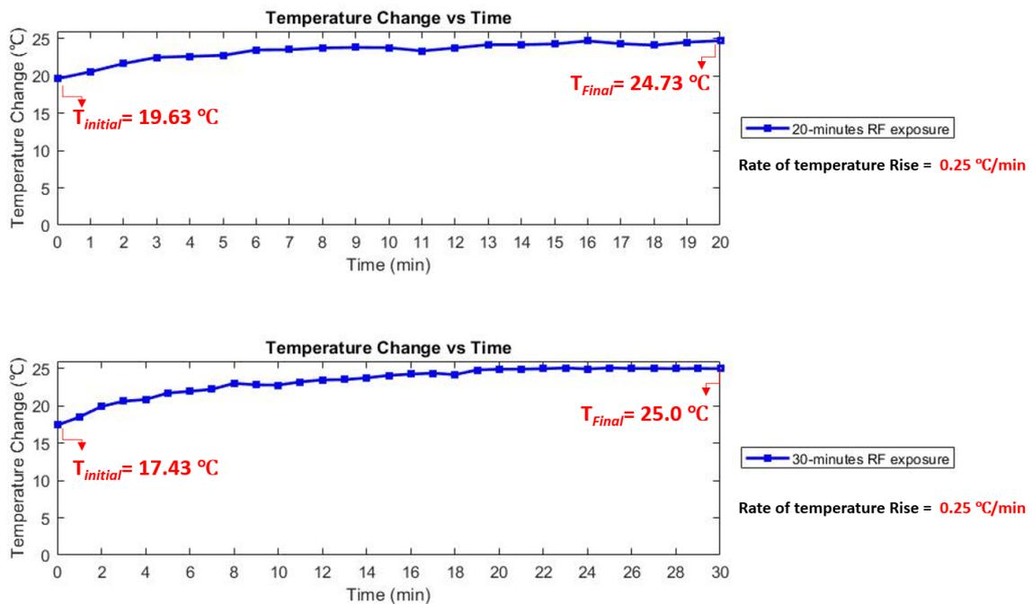
**Figure 4.** The temperature response of porcine skin to RF exposure at 26 GHz. The top image illustrates temperature variation after 20 min of exposure, while the bottom image illustrates the variation after 30 min of exposure. Temperature measurements were captured using an IR camera, with three readings per minute averaged to reduce uncertainty. The rate of temperature rise was determined by calculating the slope between the first and last data points.
