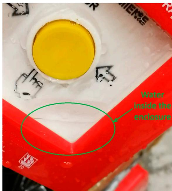
**Figure 19.** A view of a sample no. 36 of the FCB activating device after testing the degree of protection of the enclosure (IP54 enclosure rating); negative test result, and water entered the enclosure and prevented the proper operation (green circle).
