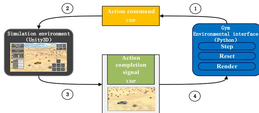
Figure 4. Bidirectional communication mechanism.
