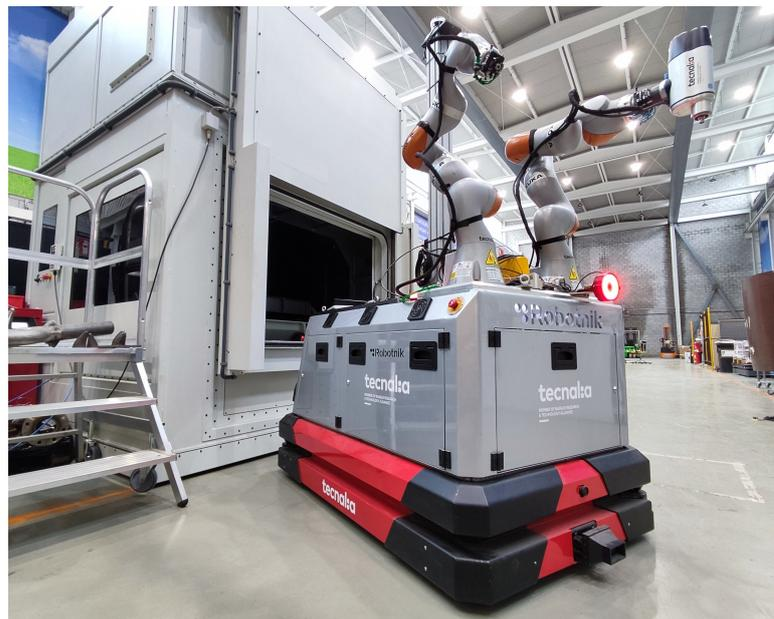
**Figure 6.** Mobile manipulator used for the implementation of the mobile visual servoing architecture.
