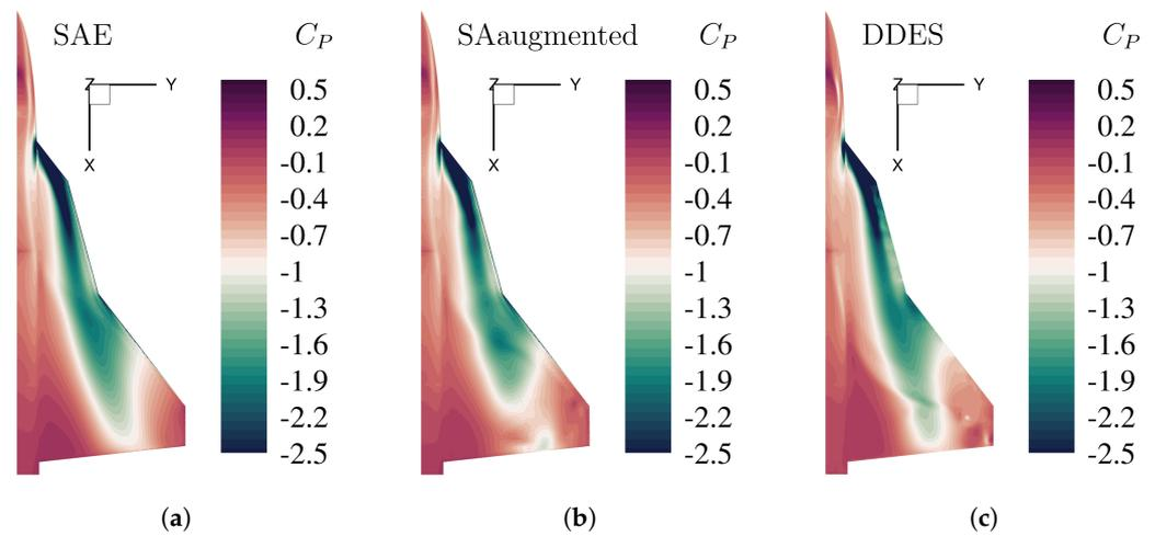
**Figure 8.** Surface pressure distribution by the means of pressure coefficient  $C_P$  at Mach number  $M_\infty = 0.15$ , Reynolds number  $Re = 3 \cdot 10^6$ , and angle of attack  $\alpha = 24^\circ$ , for different numerical turbulence models. (a) Original SA model with Edwards-modification. (b) Enhanced SA model with augmented model coefficients (Table 3). (c) High-fidelity DDES reference simulation.
