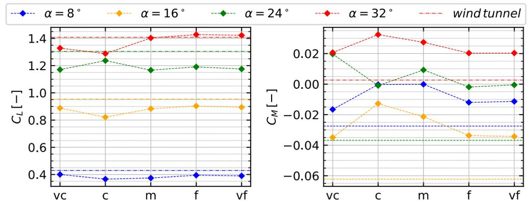
**Figure 2.** Gridstudy of a generic double delta wing. Lift coefficient  $C_L$  and pitching moment coefficient  $C_M$  for five grid resolution at angles of attack  $\alpha = [8^\circ; 16^\circ; 24^\circ; 32^\circ]$ . Grid levels: vc—very coarse; c—coarse; m—medium; f—fine; and vf—very fine.
