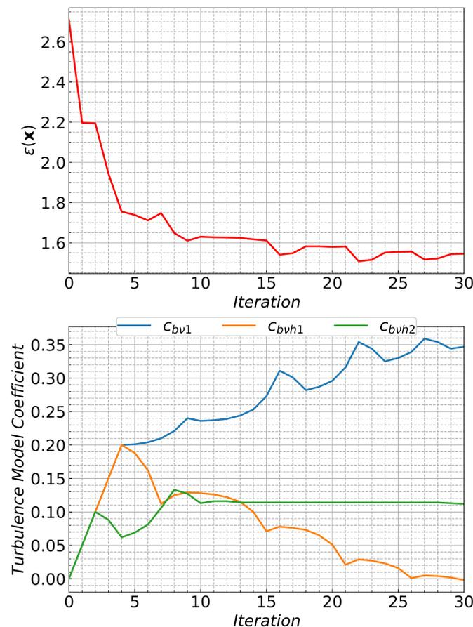
**Figure 6.** Sample optimization results. In the top part, the objective function  $\mathcal{E}(x)$  (Equation (5)) versus optimization iterations is shown. In the lower part, the corresponding turbulence model coefficients are plotted.
