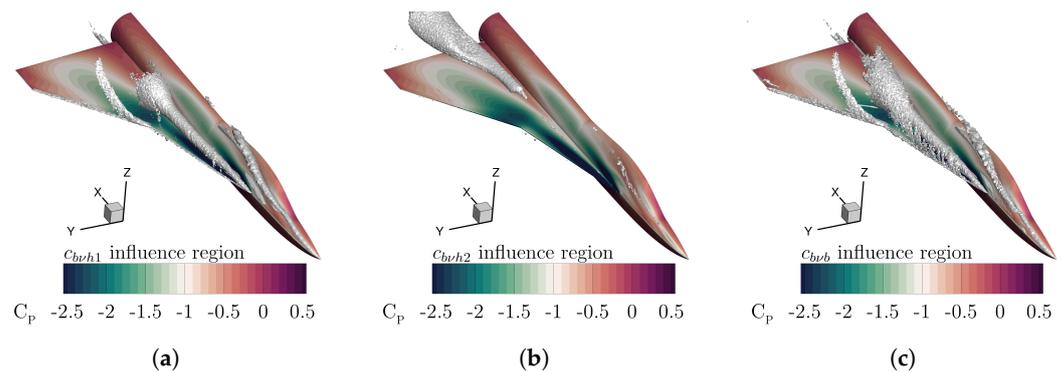
**Figure 4.** Influence regions of the additional turbulence model coefficients. (a)  $c_{bv/h1}$  acts on fully developed vortices upstream of vortex breakdown. (b)  $c_{bv/h2}$  influences mainly regions downstream of the vortex breakdown. (c)  $c_{bv/b}$  acts in proximity the vortex breakdown.
