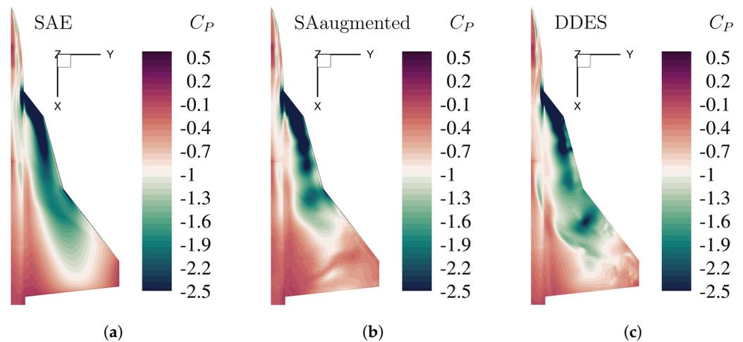
**Figure 9.** Surface pressure distribution by the means of pressure coefficient  $C_P$  at Mach number  $M_\infty = 0.15$ , Reynolds number  $Re = 3 \cdot 10^6$ , and angle of attack  $\alpha = 32^\circ$ , for different numerical turbulence models. (a) Original SA model with Edwards-modification. (b) Enhanced SA model with augmented model coefficients (Table 3). (c) High-fidelity DDES reference simulation.
