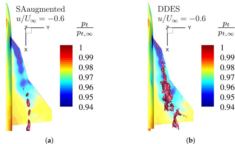
**Figure 16.** Detailed reverse flow regions by an isosurface of the non-dimensional axial velocity  $u/U_\infty \leq -0.6$  at Mach number  $M_\infty = 0.15$ , Reynolds number  $Re = 3 \cdot 10^6$ , and angle of attack  $\alpha = 32^\circ$ , for different numerical turbulence models. Additionally, the surface total pressure ratio distribution  $p_t/p_{t,\infty}$  is shown. (a) Enhanced SA model with augmented model coefficients (Table 3). (b) High-fidelity DDES reference simulation.
