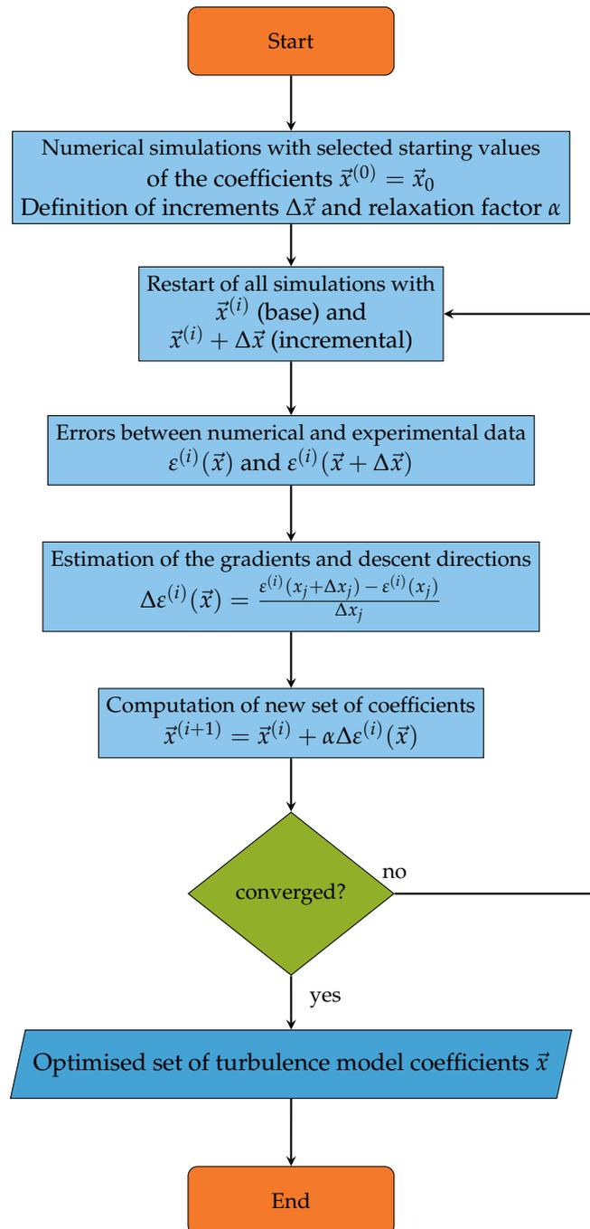
**Figure 5.** Flowchart of the coefficient optimization procedure.
