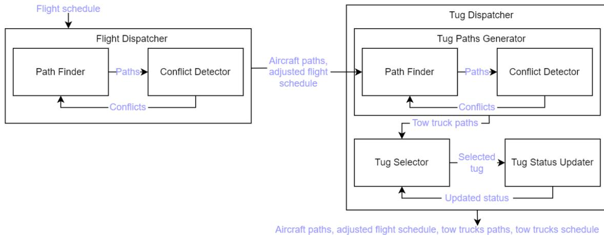
**Figure 1.** Control flow of the algorithm.
