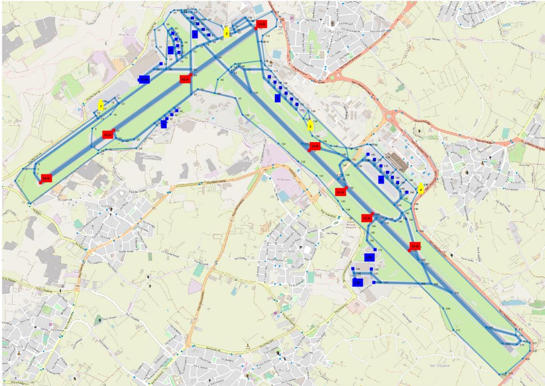
**Figure 2.** Directed graph for Malta International Airport (MLA) superimposed on MLA graphical representation. The thickness of the lines represents the runways (thickest), taxiways (medium thickness) and service roads (thinnest). The blue nodes represent the aircraft stands, the red nodes mark the ToPs/LEPs and the yellow nodes show the position of the tow truck depots.
