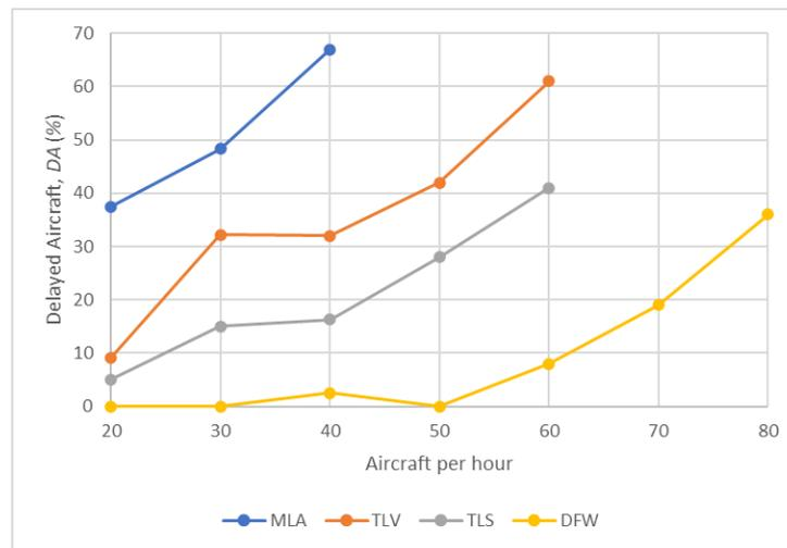
**Figure 4.** Delayed aircraft, DA (%), in Test Scenario 1.
