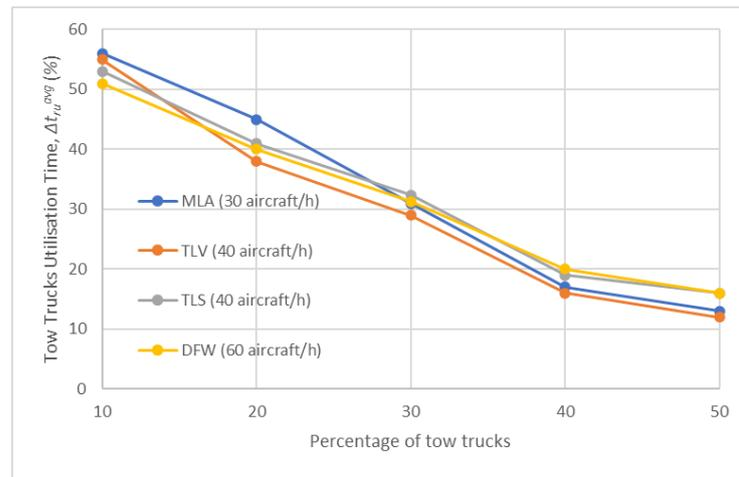
Figure 14. Tow truck utilisation time,  $\Delta t_{ru}^{avg}$  (%), in Test Scenario 4.
