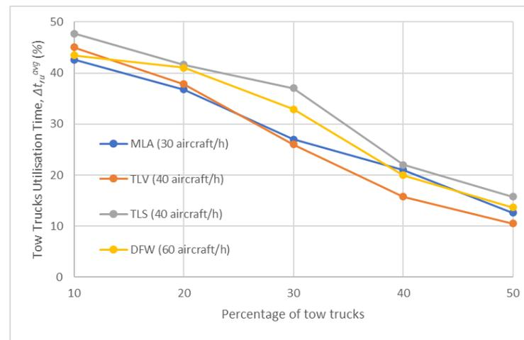
Figure 11. Tow truck utilisation time,  $\Delta t_{ru}^{avg}$  (%), in Test Scenario 3.
