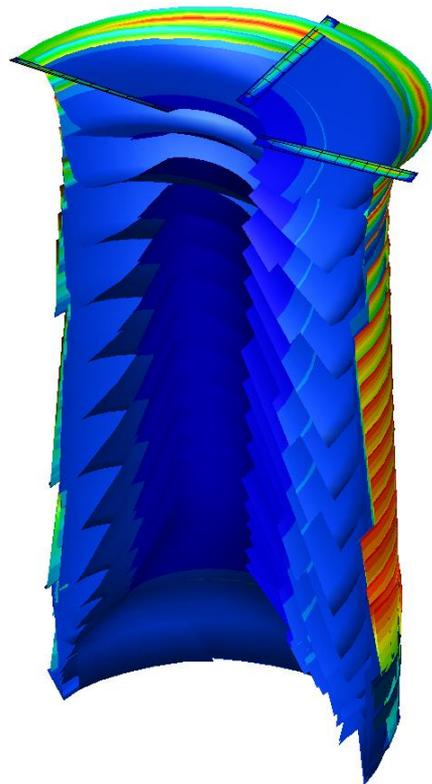
**Figure 8.** Free-wake structure in hover,  $C_T/\sigma = 0.16$ . The colors represent the trailed vorticity strength. Red = tip vortex with high positive vorticity, blue = inboard vorticity with moderate to low negative values.
