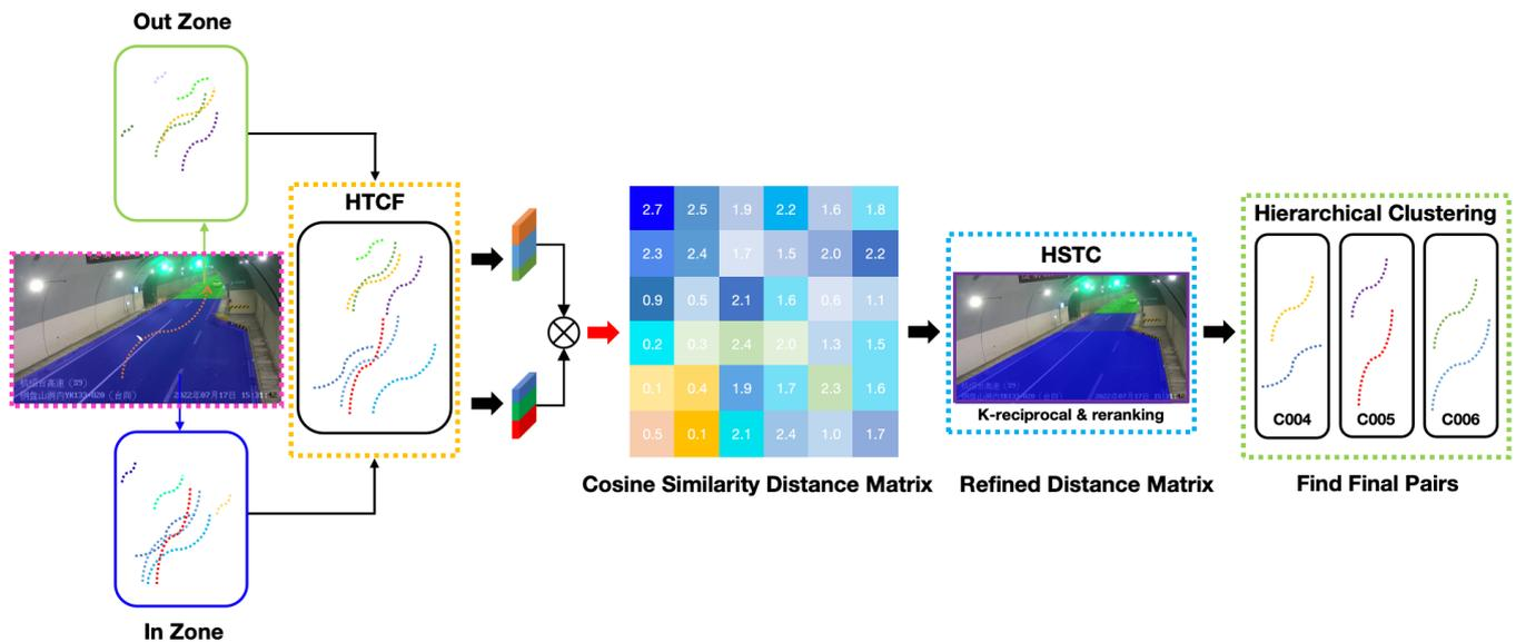
**Figure 8.** Cross-camera candidate trajectories matching process. The red-boxed image represents single-camera entry and exit trajectory processing, the yellow-boxed module represents the candidate trajectory filtering, while the blue-boxed image and green-boxed stage respectively represent the spatio-temporal constraint module for overlapping fields of view and trajectory clustering across adjacent cameras.
