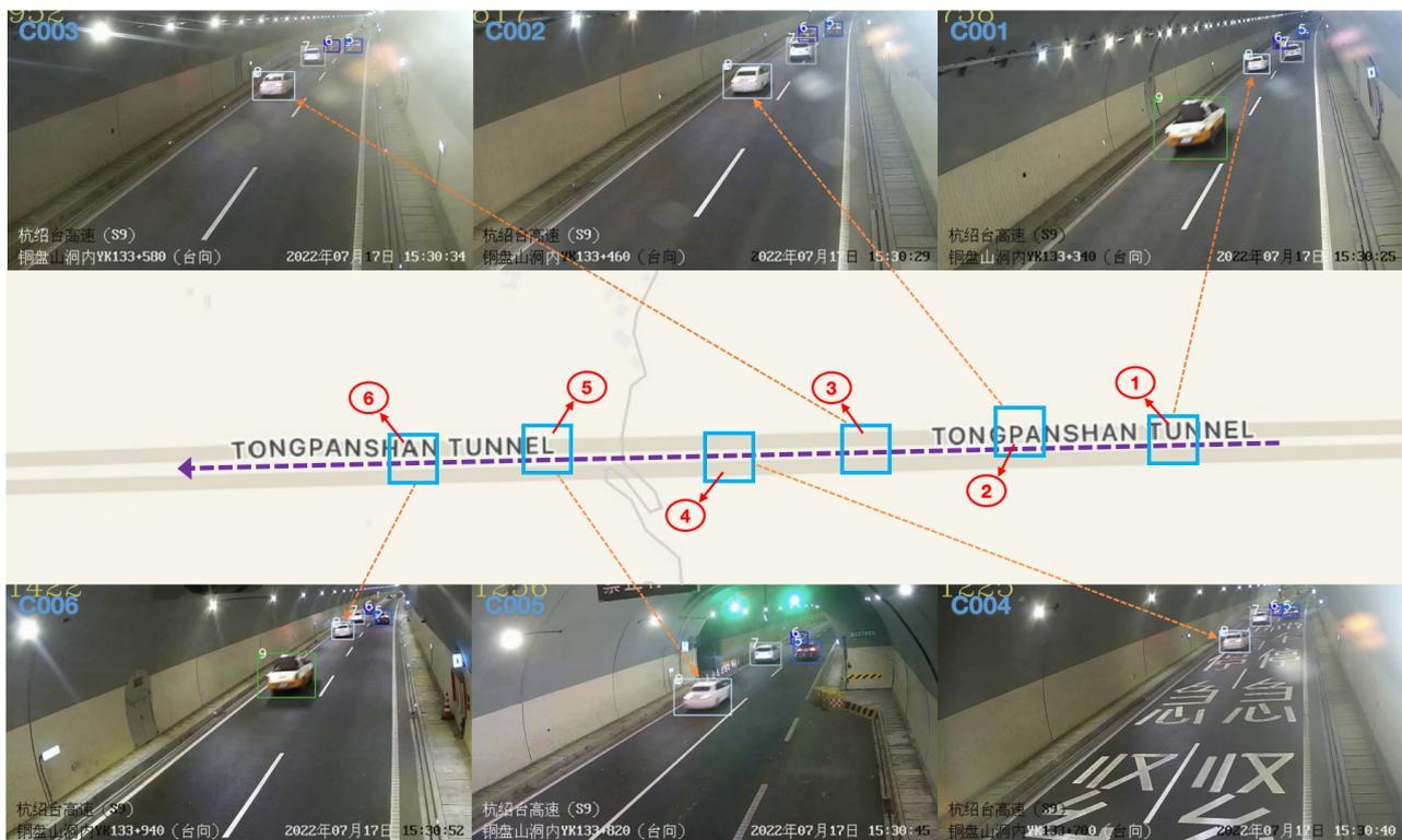
**Figure 1.** Illustration of Multi-Camera Multi-Vehicle Tracking (MCMVT) task. The second row is the camera position distribution map in the scene of the Tongpan Mountain Highway Tunnel. Vehicles with IDs 5, 6, 7, 8, and 9 are correctly tracked by multiple cameras, and a visualization tracking chain is presented for the vehicle with ID 8. “C00X” represents the camera ID.
