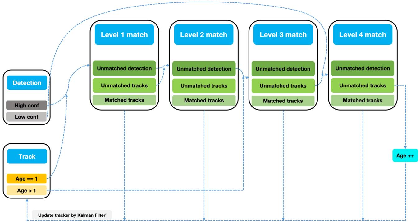
**Figure 6.** Cascade Multi-Level Multi-Target Tracking association.
