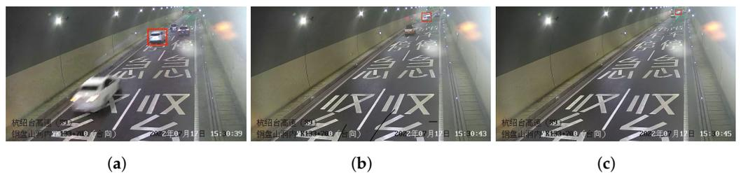
**Figure 4.** Illustration of target scale variation of vehicles in near, medium, and far field of view. In (a–c), the vehicles highlighted in red boxes represent high confidence with no occlusion, high confidence with slight occlusion, and low confidence with severe occlusion, respectively.
