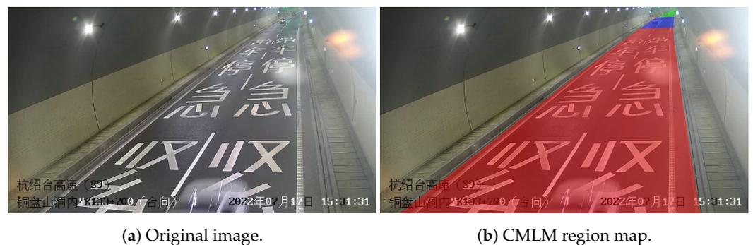
**Figure 5.** Multi-level field of view illustration. The CMLM region map indicates different intervals based on the confidence of the detection boxes, with red, blue, and green representing near, medium, and far field of view regions, respectively, and their confidence thresholds are 0.5, 0.3, and 0.1.
