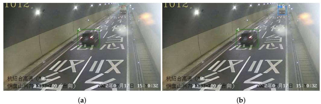
**Figure 7.** Illustration of vehicle tracking visualization before and after introduction of CMLM under the C004 camera. (a) represents before introducing CMLM, there was a situation of trajectory loss for large vehicles; (b) represents vehicle with id 19 is tracked correctly after introducing CMLM.
