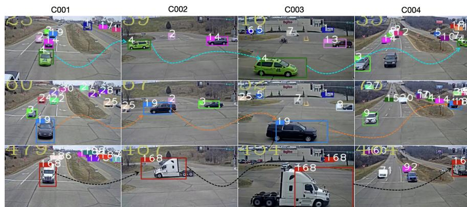
**Figure 13.** Qualitative results of MCMVT for CityFlow. From left to right, the blue, orange, and red lines with arrows represent the tracking trajectories of IDs 4, 19, and 168 under each camera.
