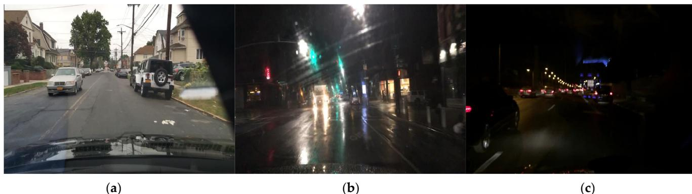
**Figure 1.** Various environments during driving: (a) lane marking is severely deteriorated; (b) lane markings are nearly erased due to rainwater; (c) lighting conditions are insufficient, making the lane markings barely visible.
