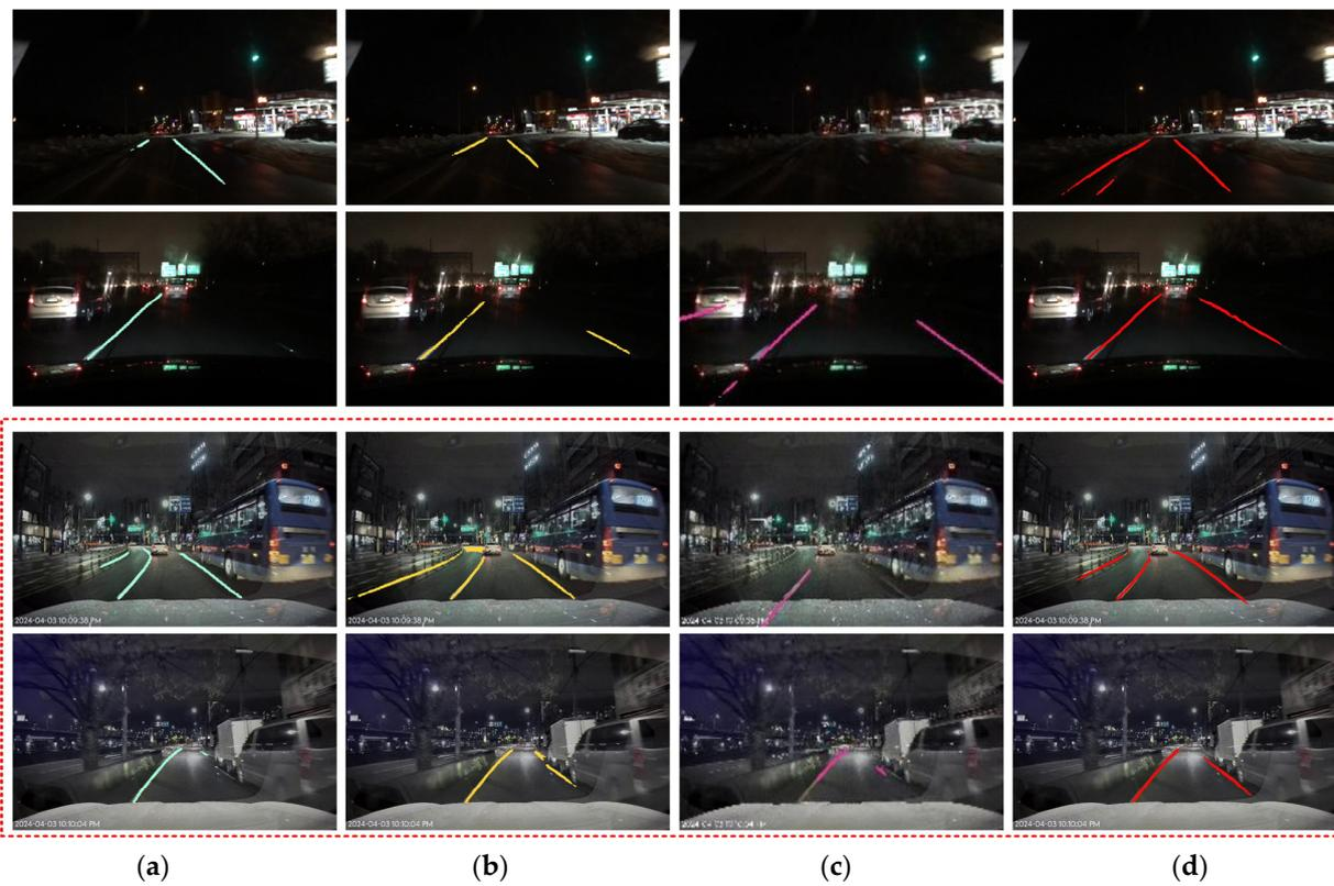
Figure 18. The result of the comparison in scenario 3 (the red dotted box represents the Lab. dataset): (a) U-Net lane detection, (b) Depthwise separable U-Net, (c) U-Net ConvLSTM, and (d) proposed method.
