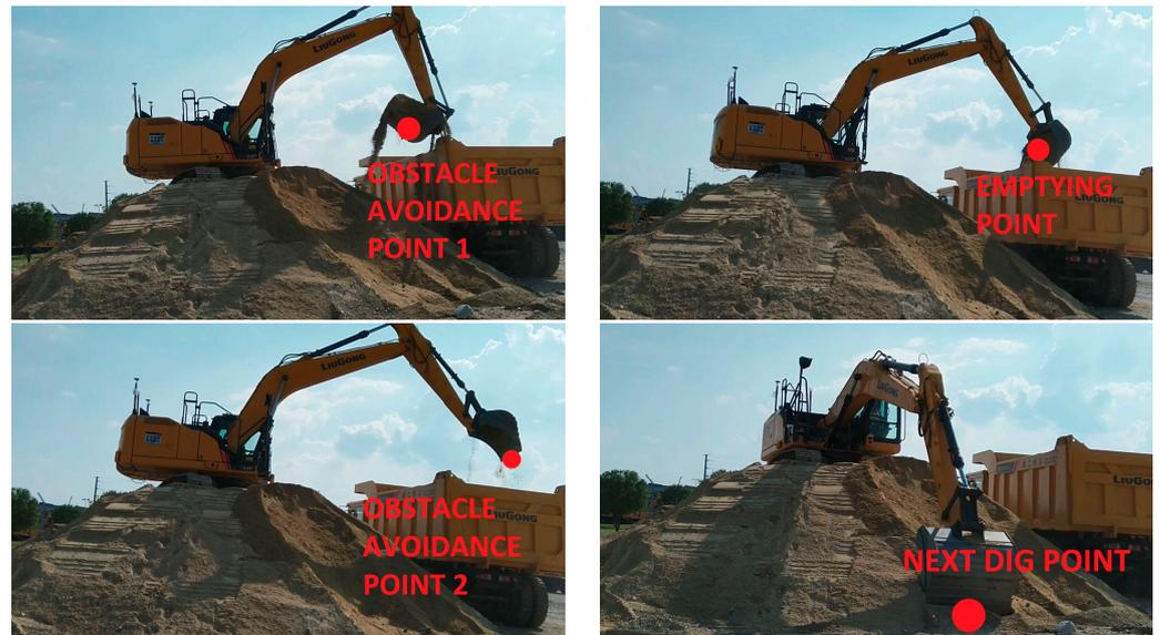
Figure 6. Diagram of six key point positions.
