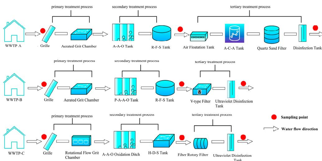
**Figure 1.** Location of wastewater sampling points in different WWTPs (A-A-O: Anaerobic-Anoxic-Oxic; P-A-A-O: Preanoxic-Anaerobic-Anoxic-Oxic; R-F-S: Radial-Flow-Sedimentation; H-D-S: High-Density-Sedimentation; A-C-A: Activated-Coke-Adsorption).
