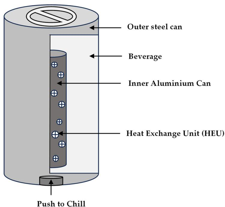
**Figure 3.** Simplified presentation of the elements of a self-cooling can with their main materials and self-cooling element. Own study based on [47].
