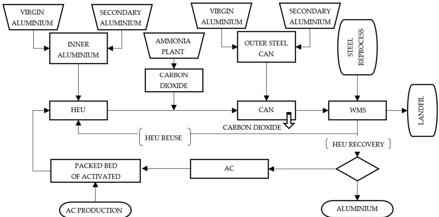
**Figure 4.** Technological process of self-cooling beverage cans. Own study based on [51].
