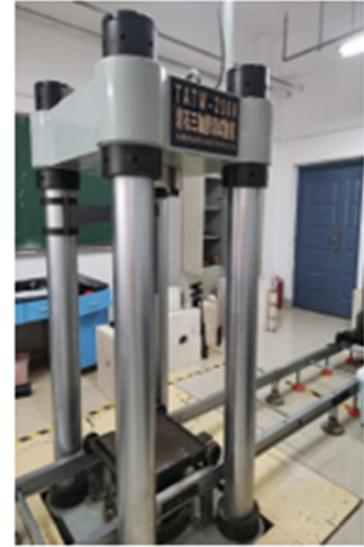
(a) Demonstration of rock sample loading (b) Rock triaxial testing machine
