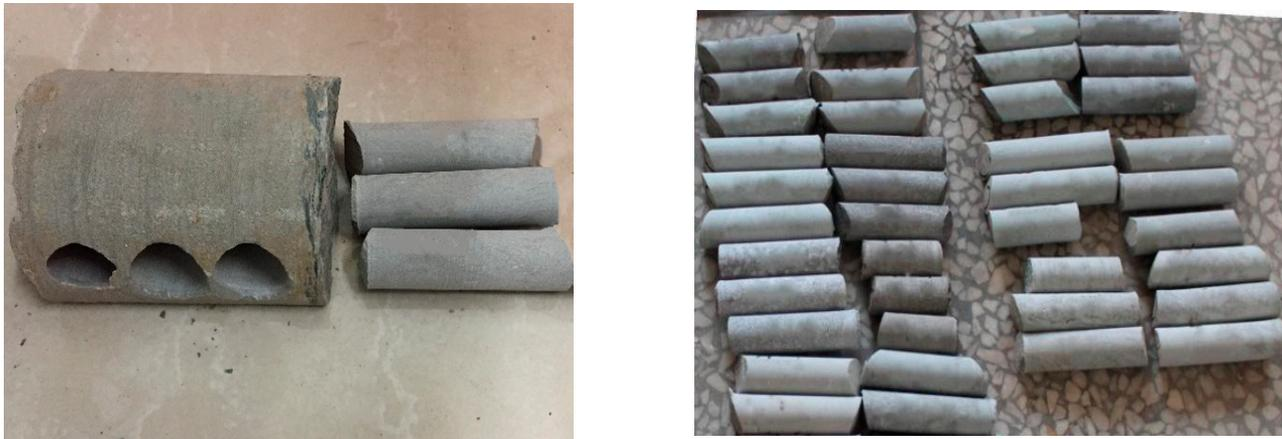
**Figure 1.** Tight sandstone core samples.
