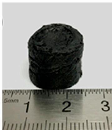
**Figure 7.** Digital image of the g-C<sub>3</sub>N<sub>4</sub>/GO aerogel. Adapted with permission from [102]. Copyright © 2017 Elsevier.
