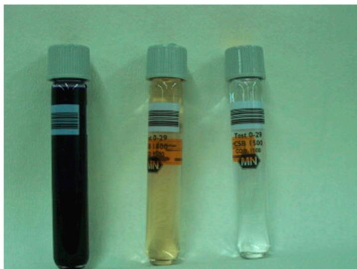
**Figure 14.** Basic Blue 41 solution (**left**) after oxidation at 450 °C (**middle**) and 600 °C (**right**). Reprinted with permission from [160]. Copyright © 2009 Elsevier.
