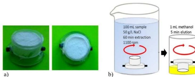
**Figure 4.** Configuration of stir FPSE device (a) along with the extraction procedure (b). Reproduced from [30] with permission of Elsevier.
