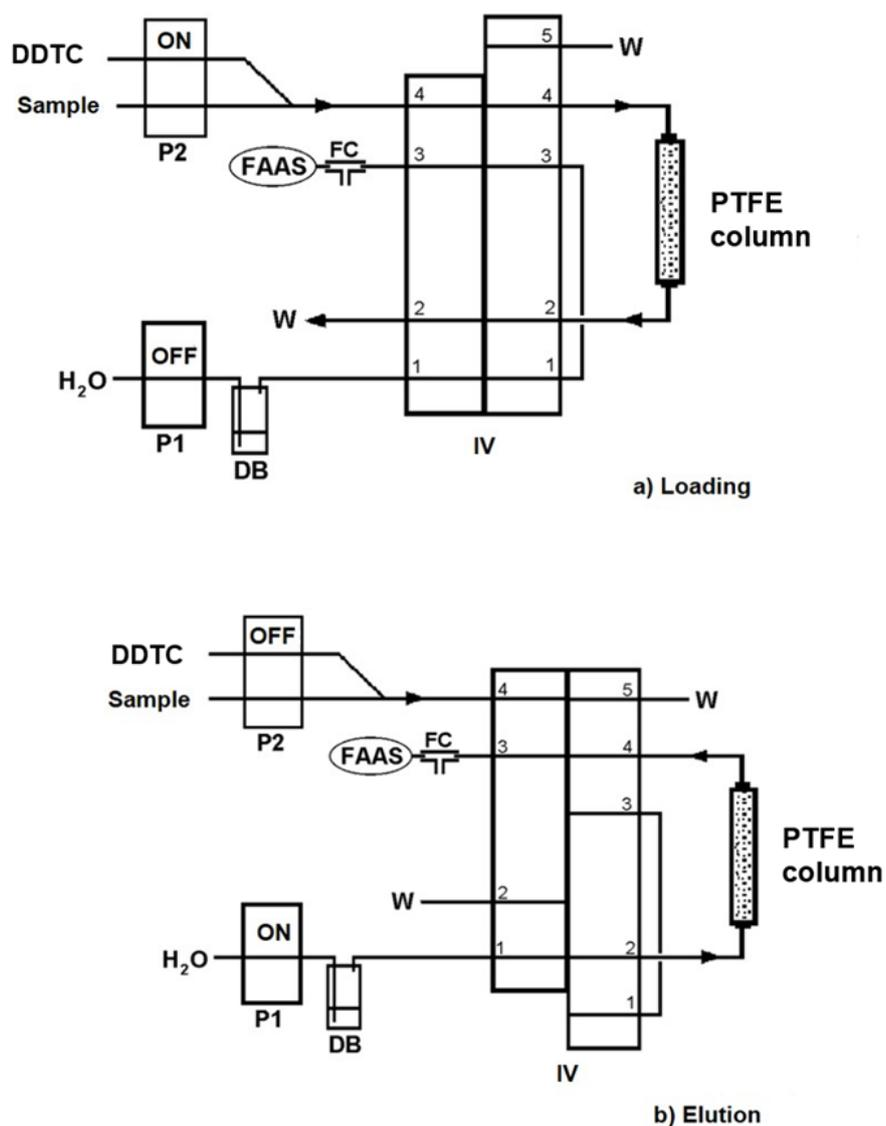
**Figure 1.** Schematic manifold of the on-line flow-injection–solid-phase extraction (FI-SPE) system coupled with flame atomic absorption spectrometry (FAAS) in (a) loading / preconcentration and (b) elution / measurement steps. P1, P2; peristaltic pumps, IV; injection valve, DB; displacement bottle, FC; flow compensation unit, W; waste.
