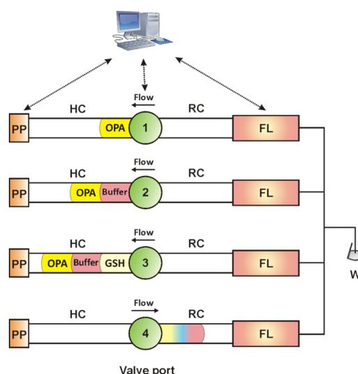
**Figure 1.** Zone fluidics (ZF) sequence and configuration: PP = pump, HC = holding coil, RC = reaction coil, FL = fluorimetric detector and W = waste (for experimental details, see Section 2.4).
