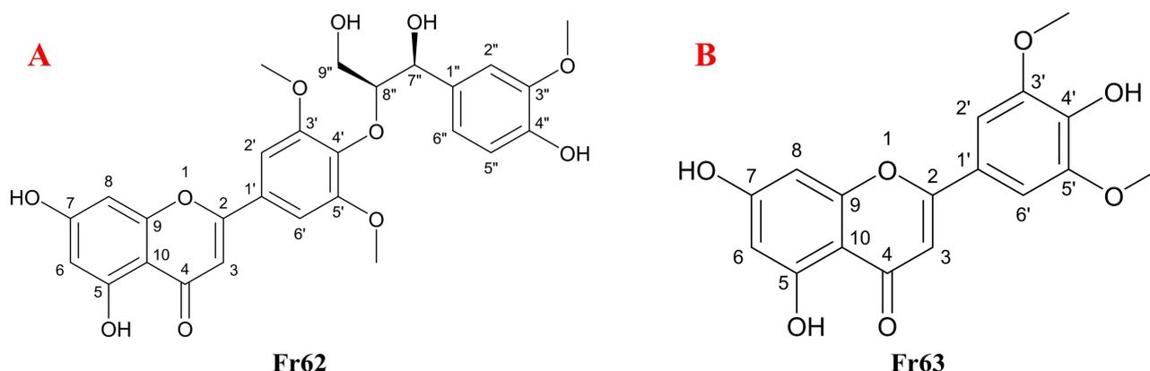
**Figure 6.** Chemical structures of the isolated DPPH inhibitors. (A,B) represent the chemical structure of Fr62 and Fr63, respectively.
