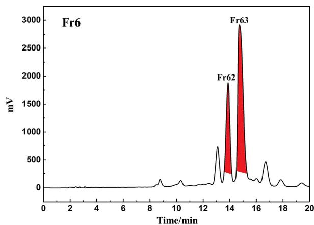
**Figure 4.** The preparative chromatogram of the *E. nutans* target Fr6 sample on a Kromasil 100-5-Phenyl preparative column. The red part represents the target component (Fr62 and Fr63).
