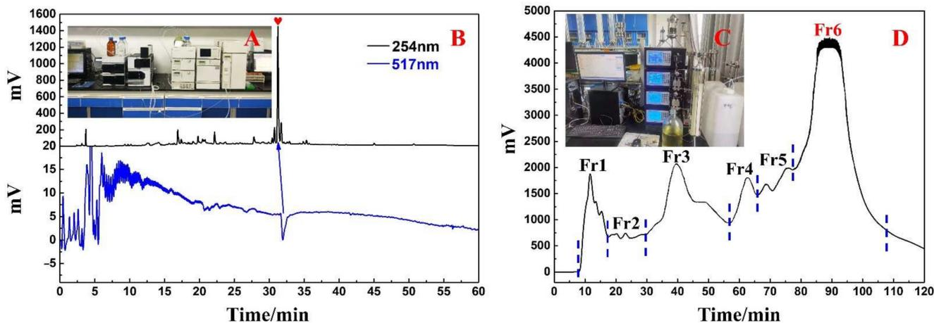
Figure 1. The actual online HPLC-DPPH system (A) and the analytical chromatogram on a Odyssey C18 analytical column and DPPH inhibitory activity profile of the *E. nutans* crude sample (B). The actual micro gel chp20p medium pressure liquid chromatography system (C) and *E. nutans* amorphous silica gel mixture separation chromatogram (D).
