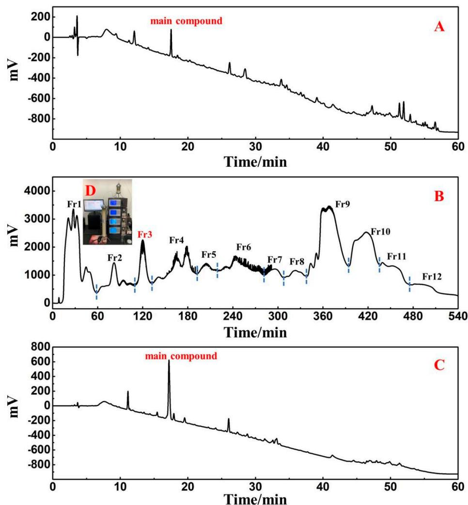
**Figure 1.** (A) The analytical chromatogram of crude *Medicago sativa* sample on the ReproSil–Pur C18 AQ analytical column. (B) The crude extract chromatogram of medium-pressure liquid chromatography pretreatment with MCI GEL<sup>®</sup> CHP20P as the stationary phase. (C) The analytical chromatogram of fraction Fr3 on the ReproSil-Pur C18 AQ analytical column. (D) The actual MCI GEL<sup>®</sup> CHP20P medium-pressure liquid chromatography system.
