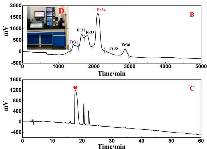
**Figure 2.** (A) The analytical chromatogram of fraction Fr3 on the ReproSil–Pur C18 AQ analytical column. (B) The fraction Fr3 chromatogram of medium-pressure liquid chromatography pretreatment with Sephadex LH-20 as the stationary phase. (C) The analytical chromatogram of fraction Fr34 on the ReproSil-Pur C18 AQ analytical column. (D) The actual Sephadex LH-20 medium-pressure liquid chromatography system.
