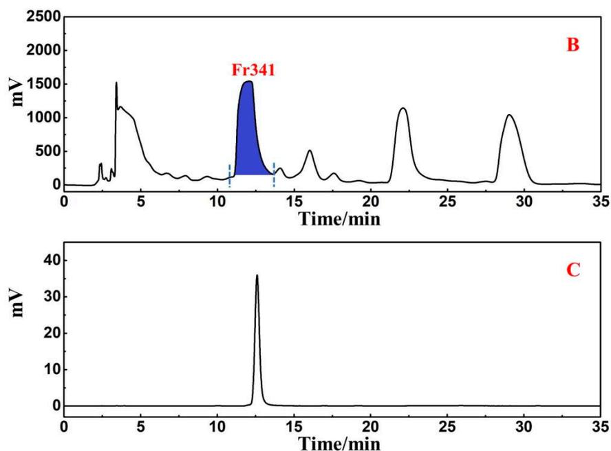
**Figure 3.** (A) The analytical chromatogram of fraction Fr34 on the ReproSil-Pur C18 AQ. (B) High-pressure preparative fraction Fr34 chromatogram using a ReproSil-Pur C18 AQ preparative column. (C) The analytical chromatogram of fraction Fr341 on the ReproSil-Pur C18 AQ.
