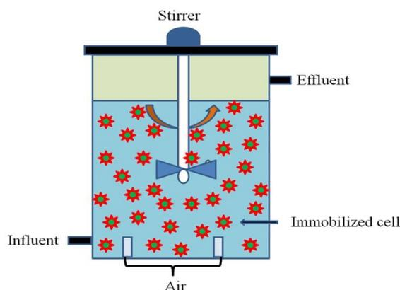
**Figure 6.** Immobilized cell bioreactor for dye removal.
