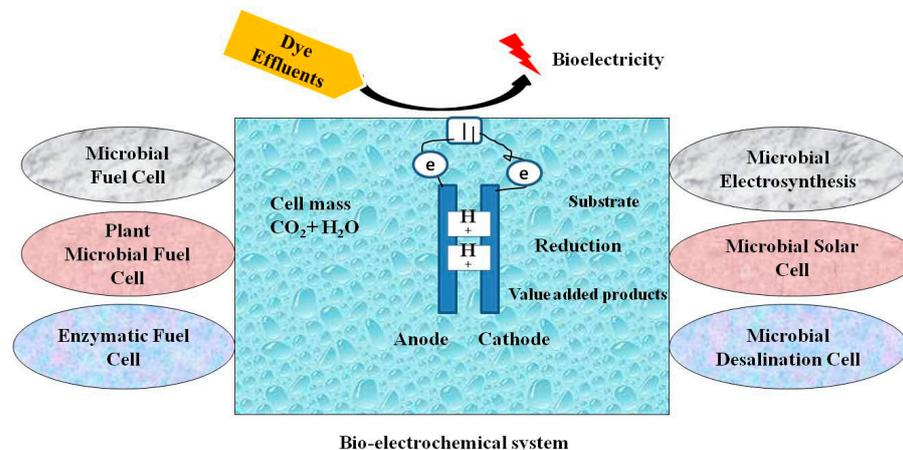
**Figure 4.** Microbial fuel cell system units.
