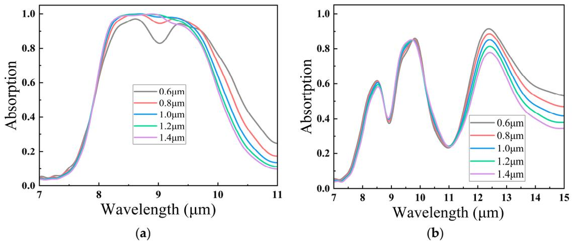
Figure 6. (a) Absorption curves of different  $l_2$  under Ex polarization; (b) absorption curves of different  $l_2$  under Ey polarization.
