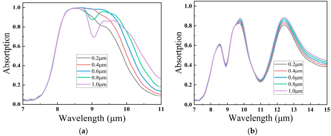
**Figure 7.** (a) Absorption curves of different  $l_3$  under Ex polarization; (b) absorption curves of different  $l_3$  under Ey polarization.
