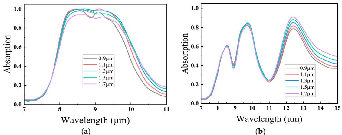
**Figure 8.** (a) Absorption curves of different  $h_2$  under Ex polarization; (b) absorption curves of different  $h_2$  under Ey polarization.
