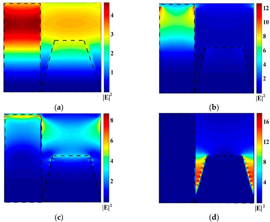
Figure 3. Electric fields at different operating wavelengths. (a) The electric field at a wavelength of 7.5  $\mu\text{m}$ ; (b) an electric field at a wavelength of 8  $\mu\text{m}$ ; (c) an electric field at a wavelength of 8.6  $\mu\text{m}$ ; (d) the electric field at the wavelength of 9.7  $\mu\text{m}$ .
