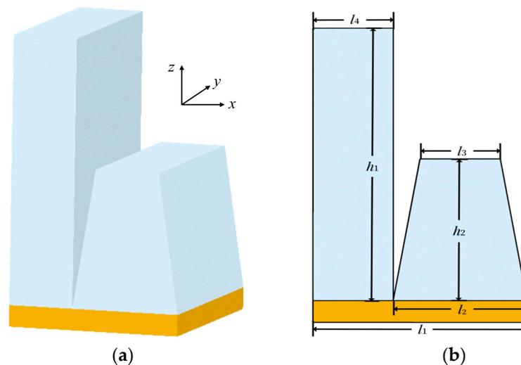
Figure 1. (a) Broadband absorber structure based on SiO<sub>2</sub>, (b) side view.
