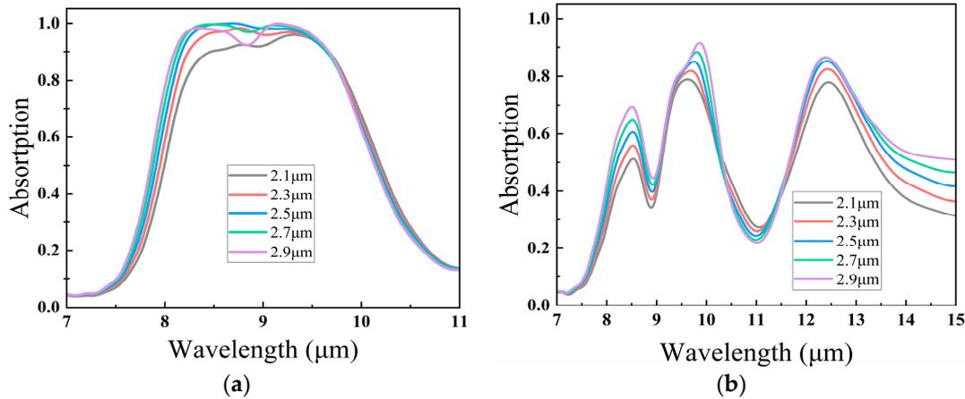
Figure 9. (a) Absorption curves of different  $h_1$  under Ex polarization; (b) absorption curves of different  $h_1$  under Ey polarization.
