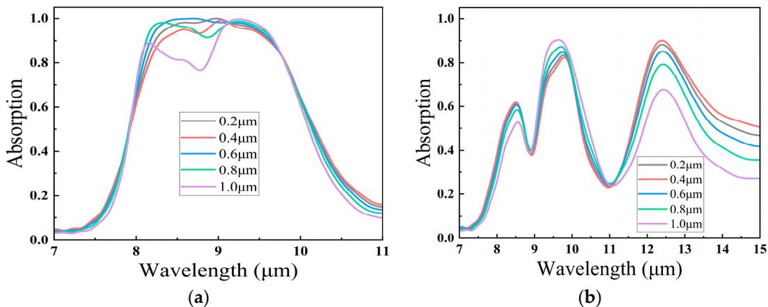
Figure 10. (a) Absorption curves of different  $l_4$  under Ex polarization; (b) absorption curves of different  $l_4$  under Ey polarization.
