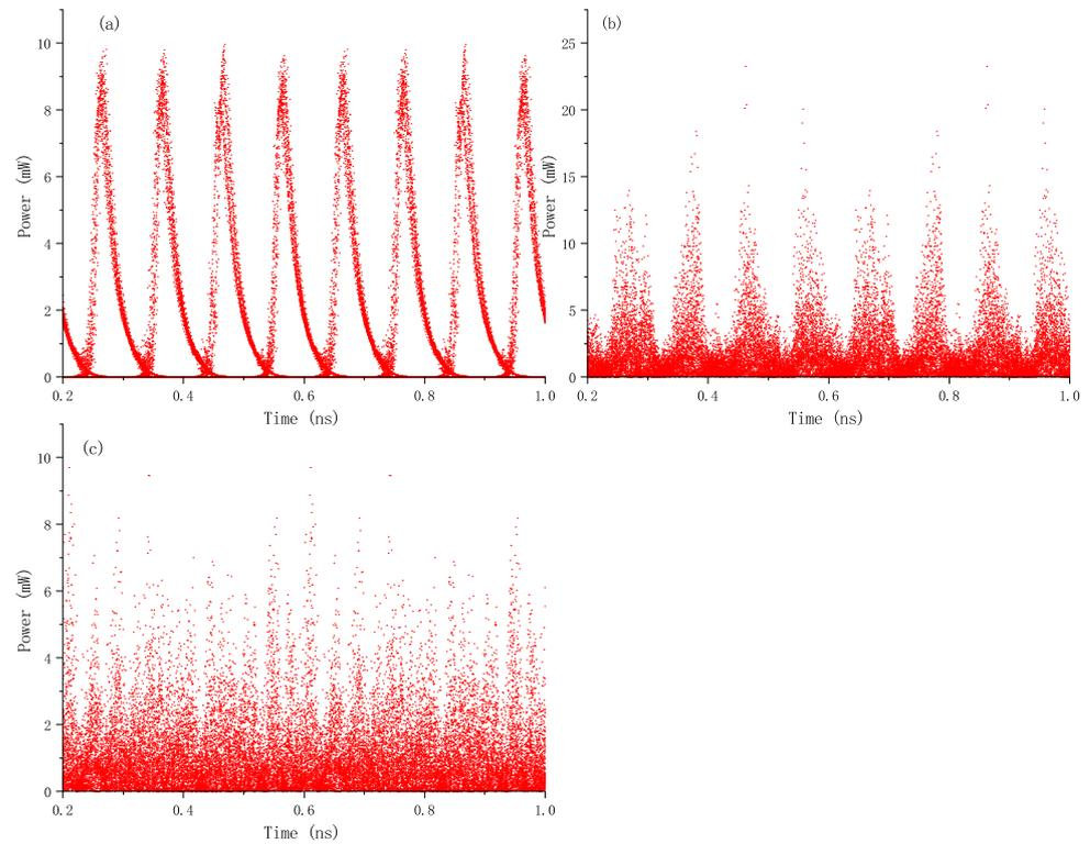
**Figure 6.** Eye diagrams of the covert channel: (a) the multiplexed optical pulses; (b) the encoded signal; and (c) the spread signal.
