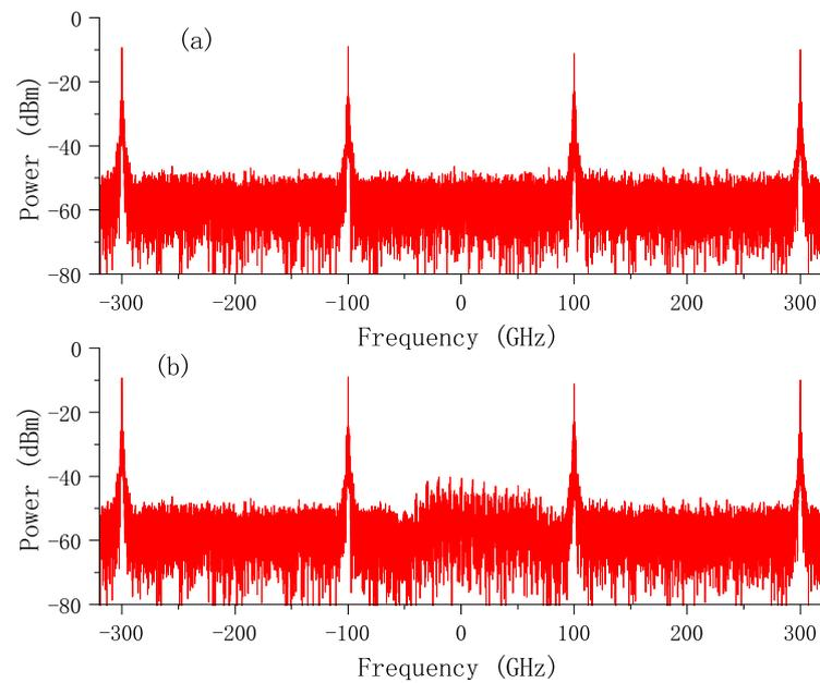
**Figure 7.** The spectrum of the public channel: (a) with the ASE noise and (b) with the optical covert signal.
