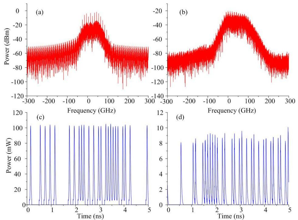
**Figure 2.** The waveform and spectrum of the optical time-division multiplexed signal. (a,c) 10 Gbps signal; (b,d) 4 time-division multiplexed 2.5 Gbps signal.
