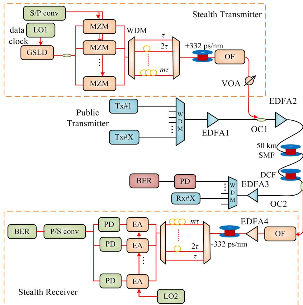
**Figure 3.** Schematic diagram of the proposed optical time-division multiplexing optical covert communication system. LO, local oscillator; S/P, serial-to-parallel; MZM, Mach–Zehnder modulator; GSLD, gain-switched laser diode; WDM, wavelength-division multiplexing; OF, optical filter; VOA, variable optical attenuator; EDFA, Erbium-doped fiber amplifier; DCF, dispersion-compensating fiber; BER, bit-error rate tester; EA, electro-absorption modulator.
