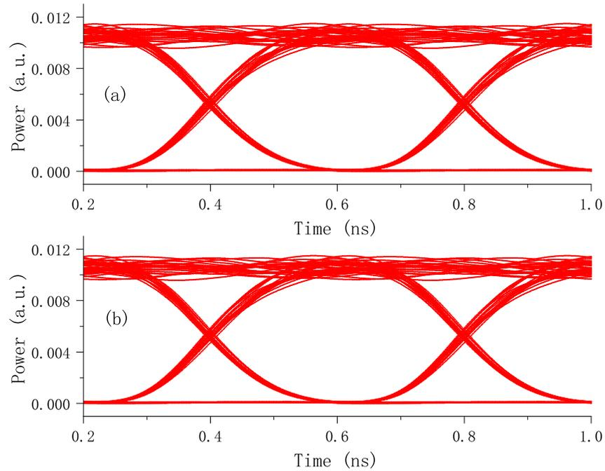
**Figure 8.** Eye diagram of the public channel: (a) with the ASE noise; and (b) with the optical covert signal.
