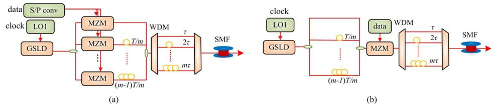
**Figure 1.** The generation of an optical time-division multiplexed optical covert signal, (a) multiple-user; (b) single-user. LO, local oscillator; MZM, Mach-Zehnder modulator; GSLD, gain-switched laser diode; WDM, wavelength division multiplexing.
