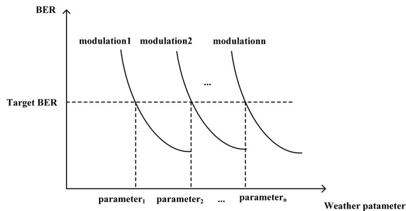
Figure 2. Optimum modulation range.
