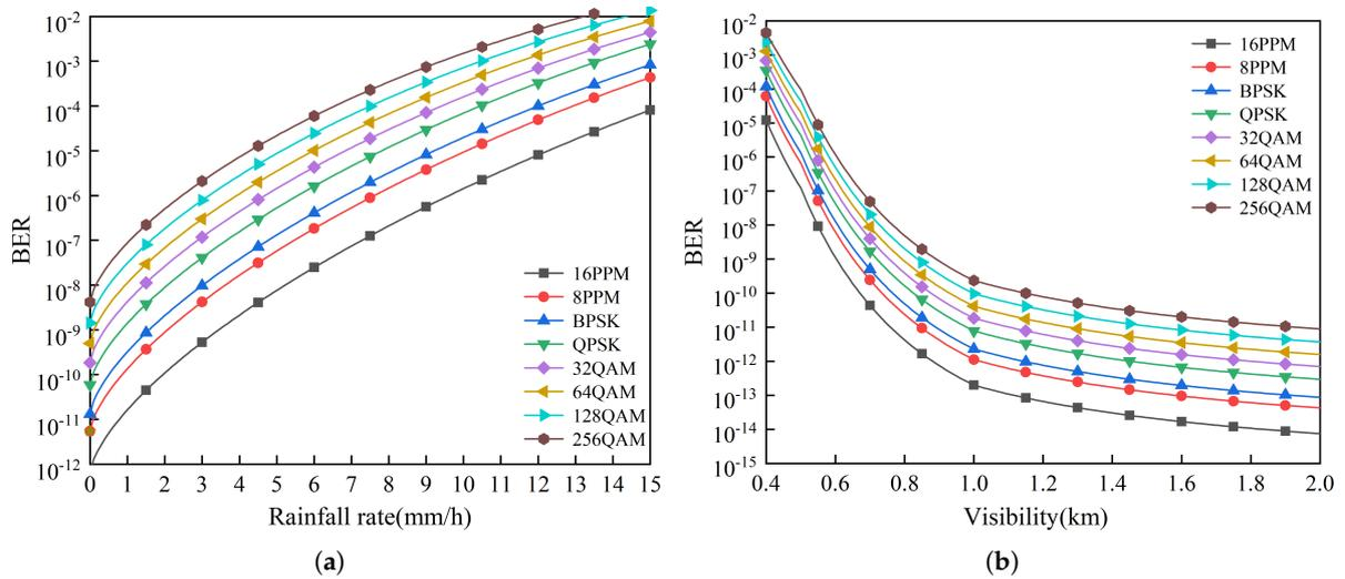
**Figure 3.** Bit error rate performance of FSO system in rainy and foggy weather condition. (a) Rainfall rate. (b) Visibility.
