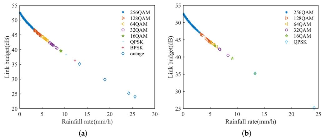
**Figure 7.** Classification of modulations for RF link in rainy weather. (a) Results of training set. (b) Results of test set.
