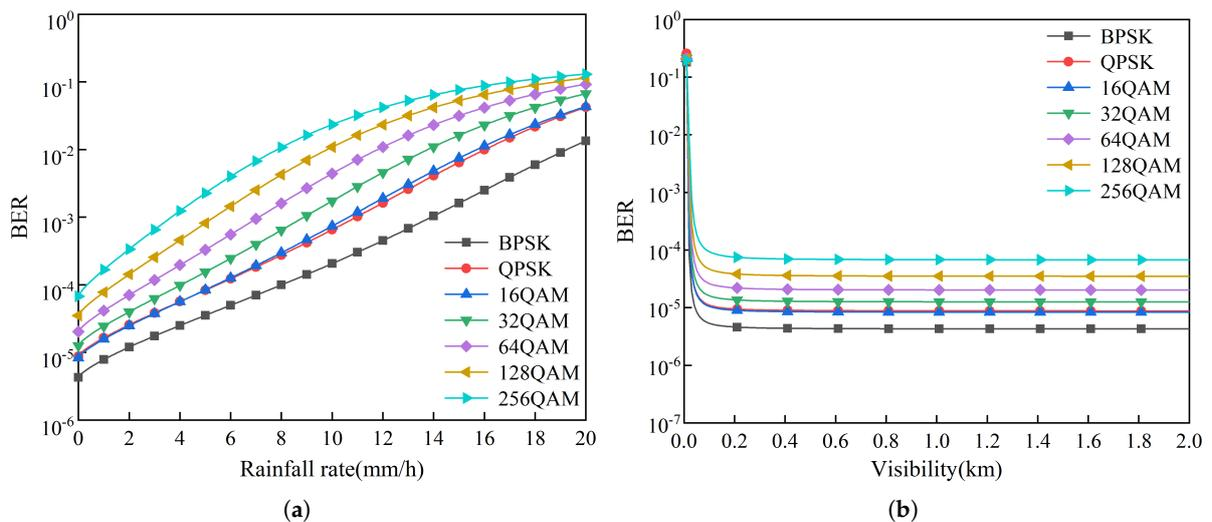
**Figure 4.** Bit error rate performance of RF system in rainy and foggy weather condition. (a) Rainfall rate. (b) Visibility.
