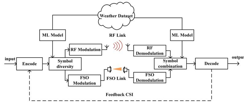
Figure 1. ML-based soft-switching model for Hybrid FSO/RF links.
