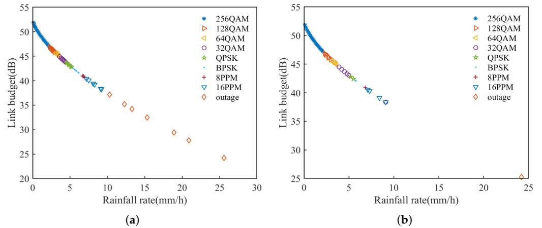
**Figure 5.** Classification of modulations for FSO link in rainy weather. (a) Results of training set. (b) Results of test set.
