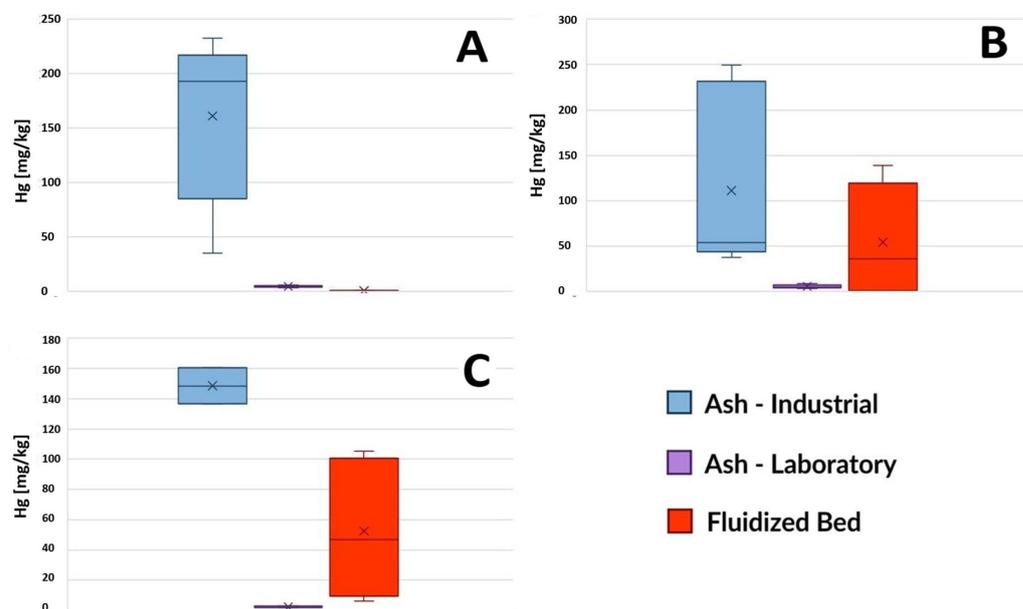
**Figure 6.** Total mercury content in ash samples from three wastewater treatment plants, based on the method of sludge incineration (laboratory furnace or industrial installation) and in disposed-of fluidized beds. (A) GOŚ Łódź, (B) Gdańsk Wschód, (C) GOŚ Dębogórze.
