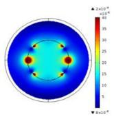
**Figure 3.** Distribution of the MRI RF magnetic field (vertically oriented) in the no material reference case within the MRI tunnel [71,72].
