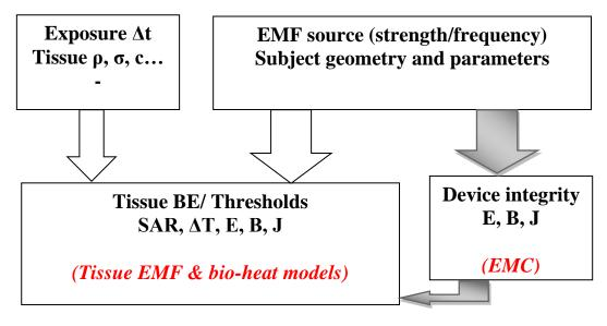
**Figure 5.** Schematics of the strategy verifying health-safety standard thresholds in body living tissues and device integrity due to interaction with EMF. Numerical used tools are indicated in red color.
