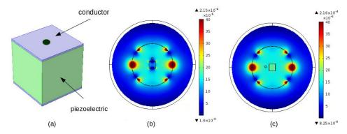
**Figure 4.** Distribution of the MRI RF magnetic field in the situation of insertion of a piezoelectric coated by electrodes (a) structure configuration, (b) distribution with electrodes perpendicular to the field, and (c) distribution with electrodes parallel to the field [71,72].
